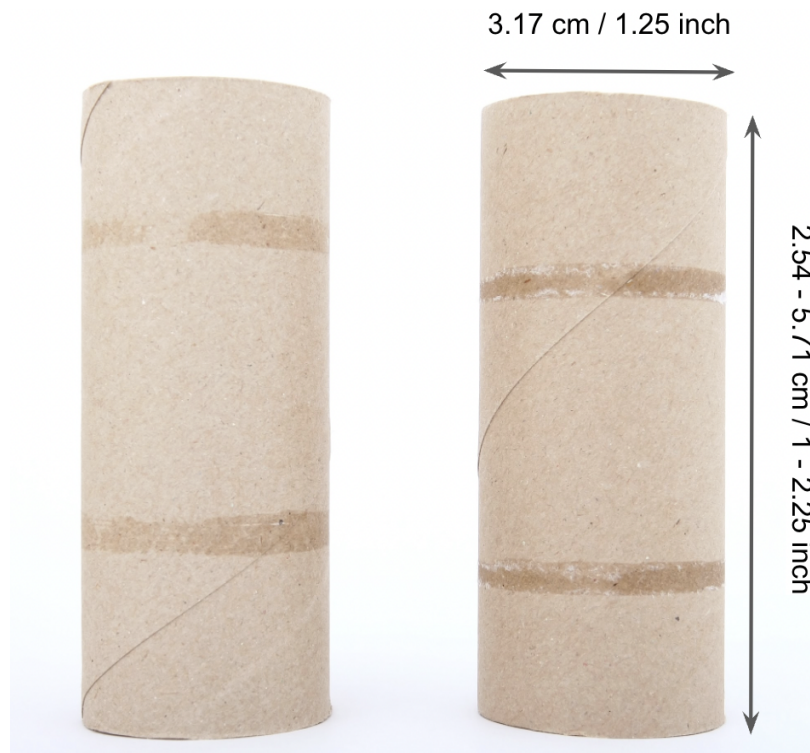
Figure 1. Identifies the toilet paper roll dimensions discussed to model a Small Parts Test Figure used to determine whether or not a toy, or a piece of a toy would be a choking hazard for the average child.
