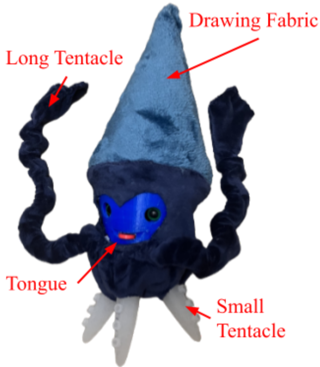
Figure 18. Our final squid design combined all the 3D printed, fabric, and silicone elements that were created during the prototyping phase. The components were joined together using either glue or sewing methods.
