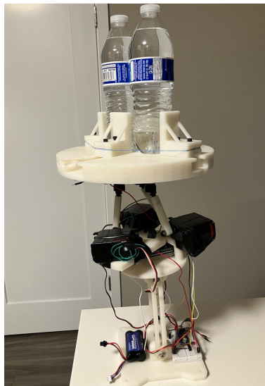
Figure 10.3. Verification test for capacity with the prototype supporting a 1kg load.
