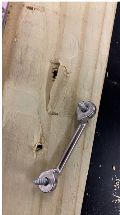
Figure 32. Fasteners used to test anchor points and straps pulled out of wood with 200 lbs of weight.
