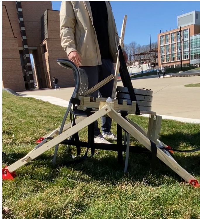
Figure 30. Insert facing downwards at a 10° angle in the 0° position loaded with 100 lbs.
