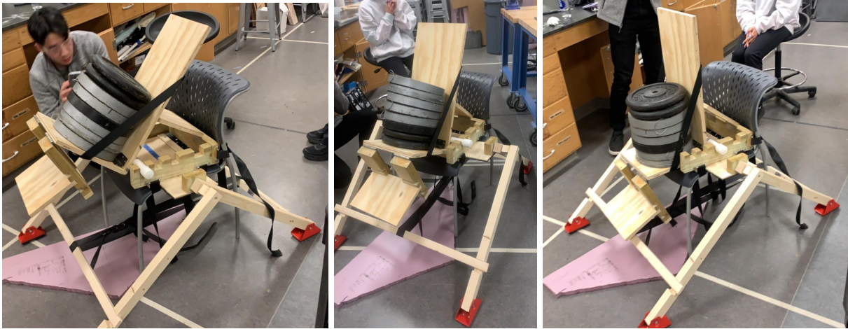
Figure 28. 200 lbs of metal plates loaded in each of the three recline positions (left: 42°, middle: 25°, right: 0°).
