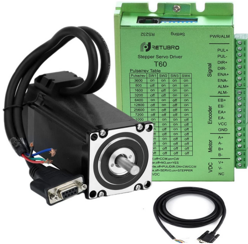
Figure 21: Nema 23 Stepper Motor w/ Driver
