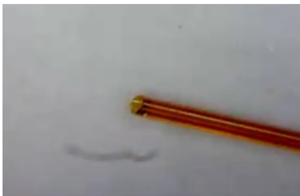
Figure A11: Roughly hand-cut capillary tube
