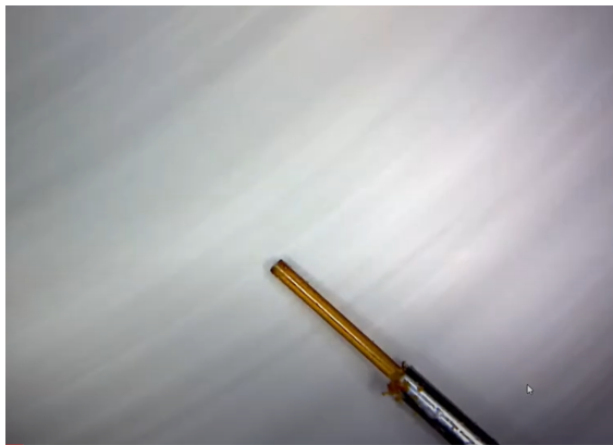
Figure 4a: Capillary Tube before grinding
