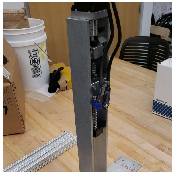
Figure 24: Build of Column with Stepper / Ball Screw Assembly
