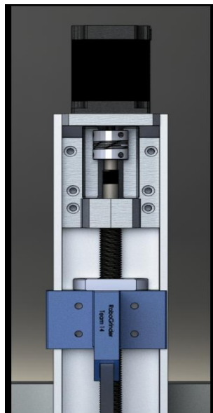
Figure 23: CAD of Column with Stepper / Ball Screw Assembly
