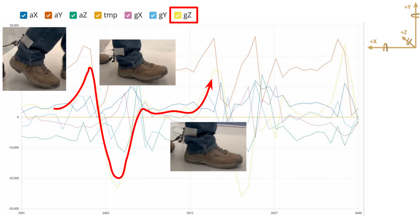
Figure 14. Angular velocity in the z-direction has a signal that clearly indicates the trend of walking.
