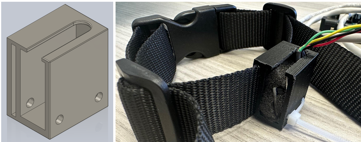
Figure 16. (Left) Sensor housing CAD model. (Right) Full housing setup to stabilize IMU and strap to the user.
