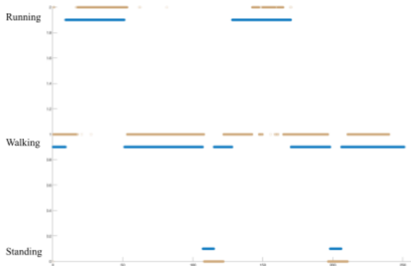
Figure 25. Plot of the algorithm state prediction compared to the actual states determined by speed and time stamped data.
