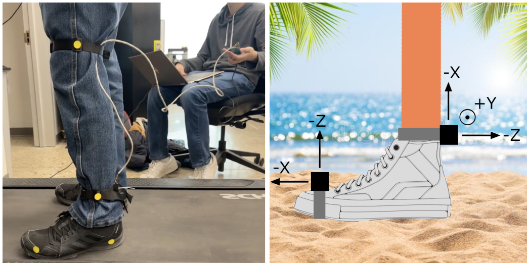
Figure 18. (Left) Data collection setup. (Right) Coordinate system of IMU sensor in relation to the user.
