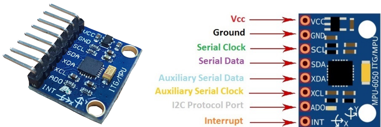
Figure C2. (Left) MPU-6050 IMU with attached pins. (Right) Pinout diagram.
