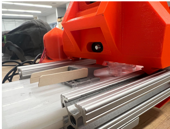
Figure 22: Initial wedge design with popsicle sticks attached to prevent stack from falling at an angle and jamming the machine.
