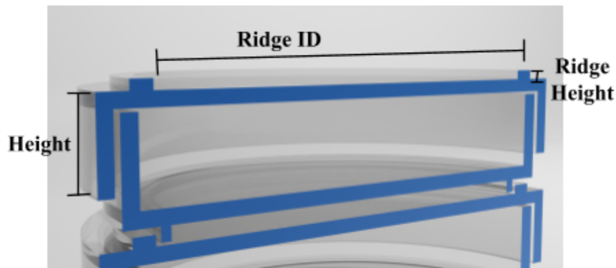
Figure 9: Dimension callouts for the plate lids
