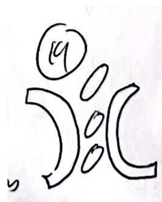
Figure A.24: Disks to allow one plate at a time through to the filling station concept.
