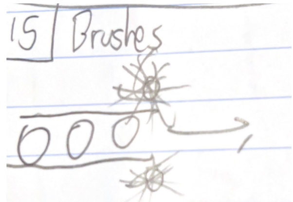
Figure A.16: Horizontal plate storage with brushes and a pushing mechanism concept
