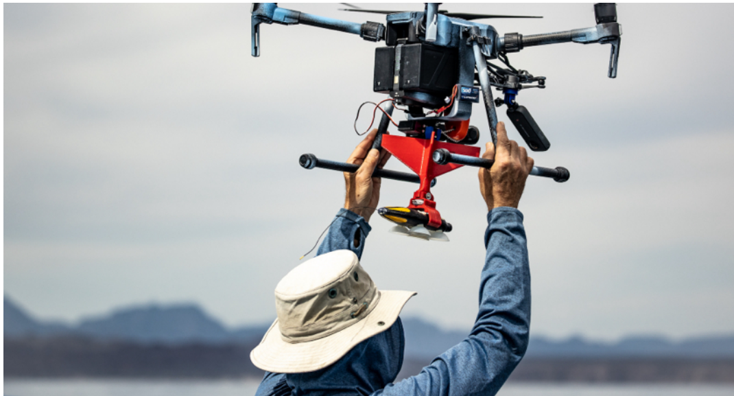
Figure 1: The current tag dropping system mounted to a drone [2]
