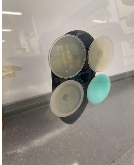
Figure 34: Fully compressed tag suction cups on polycarbonate plate
