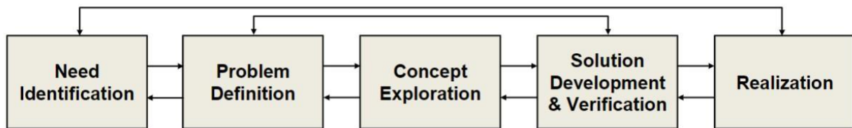
Figure 6: Standard design process model from ME450
