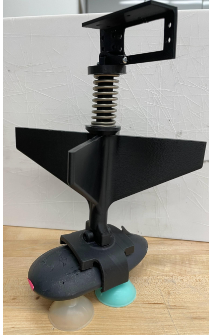
Figure 27: The assembled tag and release mechanism prior to being mounted to the test rig.
