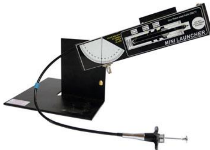
Figure 4: Spring-loaded Mini Projectile Launcher [13]
