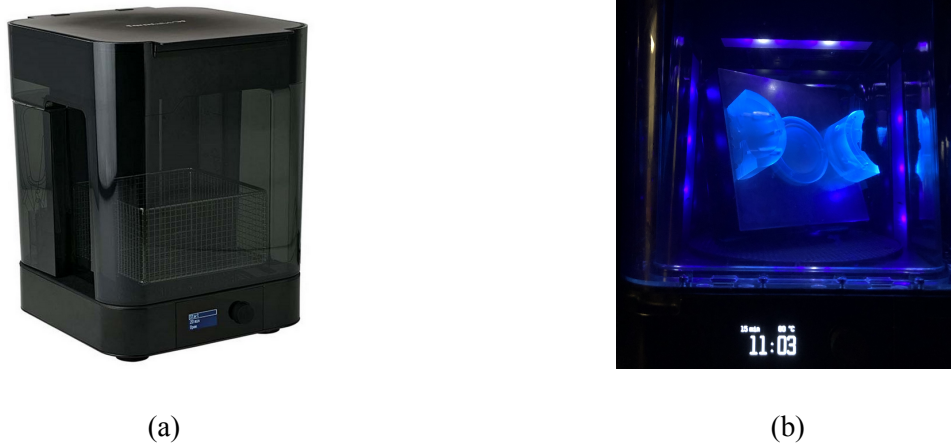
Figure 14. Automated post-processing Formlabs equipment; Formlabs Form Wash (a) and Formlabs Form Cure (b). (a) The Formlabs Form Wash was used to remove any resin from the parts that may be leftover from the 3D printing process [20]. (b) The Formlabs Form Cure was used to strengthen the parts and improve their performance which ultimately increased the quality of the suction cups made using these printed mold parts.
