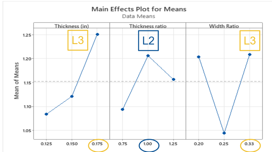
Figure 22. Main effects plot for means of vertical displacement results and the input design parameters: thickness, thickness ratio, and width ratio. The mean of means for vertical displacement data is in inches, thickness levels are in inches, and with the levels for remaining two design parameters as ratios. The combination of levels required to maximize vertical displacement is level 3, level 2, level 3 for thickness, thickness ratio and width ratio respectively. Thickness shows the most variability and therefore appears to have the most influence. Thickness and width ratio show the most variability and therefore appear to have the most influence on displacement.
