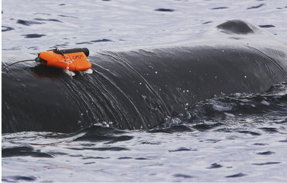
Figure 4. Attachment of Bio-logging Tag on skin of Sperm Whale Using Suction Cup Method [7]. White suction cups secure an orange bio-logging tag to the nose of a sperm whale; four cups are required per tag. The tag contains various sensors for the purpose of tracking and recording relevant cetacean information i.e., depth, sound, and movement.
