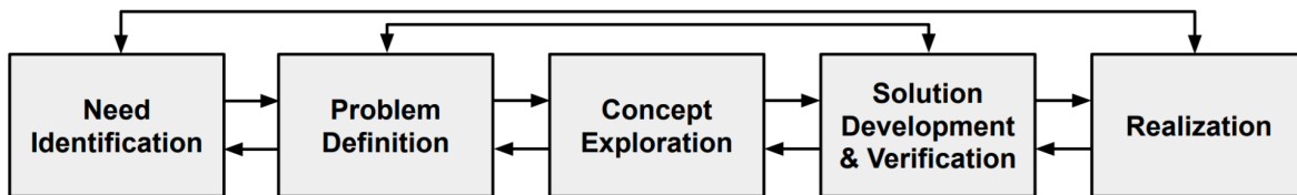
Figure 2: The ME Capstone Design Process Framework 15 . The process begins with Need Identification and after an iterative design lifecycle, ends with design Realization.
