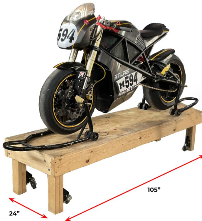
**Figure 1:** SPARK's Current Motorcycle Setup. Pictured is their current project, ATLAS, on the wood platform held in place by purchased Venom chock stands. Not pictured is the overhead winch used to lift the motorcycle from floor level onto the platform. The dimensions of the platform are shown by the red arrowheads.
