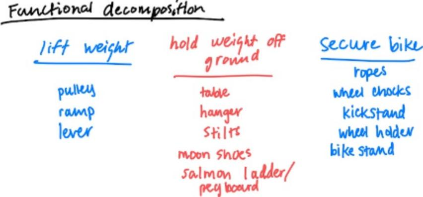
**Figure 6:** For Sarah’s iterated ideas, she first broke down the project into what she considered to be its main functions: lift weight, hold weight off ground, and secure bike.
