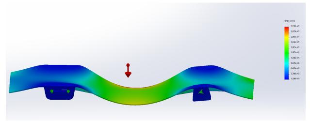
Figure 21: This figure shows the deflection of the final table surface design. The maximum deflection is about 0.3 mm.
