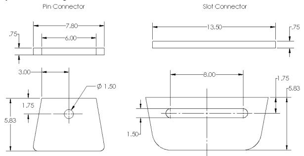
**Figure C:** Various Surface Connection fixtures. On the left is a pin connector used for one set of the scissor arm connections. On the right is a slot connector. This is used for the remaining set of scissor arm connections and allows for more free ranges of motion. Note that the features defined in this drawing are not exhaustive, but rather highlight the more critical dimensions for reference.
