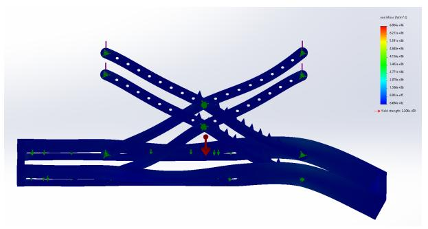
**Figure 24:** The stresses experienced by the scissor arm and base in the high position. The maximum stress is about 6 MPa which is much lower than the yield stress of 220 MPa.
