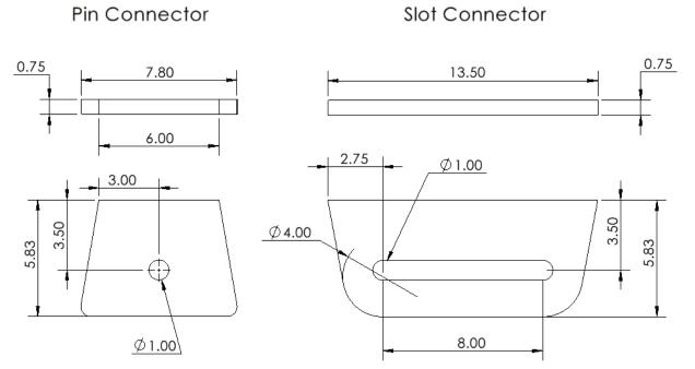
**Figure 29:** Various Surface Connection fixtures. On the left is a pin connector used for one set of the scissor arm connections. On the right is a slot connector. This is used for the remaining set of scissor arm connections and allows for more free ranges of motion. Note that the features defined in this drawing are not exhaustive, but rather highlight the more critical dimensions for reference.
