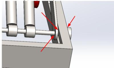
B. Cross the scissor arms with the respective joining axles in the middle. Similarly, place the table slider components with their respective axle towards the top of each scissor arm.
