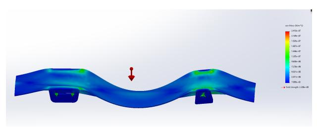
Figure 20: Stress of the final table surface design. The maximum stress is about 24 MPa which is well below the yield stress of 220 MPa.
