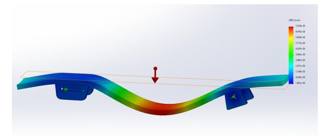
**Figure 17:** Deflection of the table surface with the Pin Axle 20 inches from the end of the table. The maximum deflection is about 0.02 mm.
