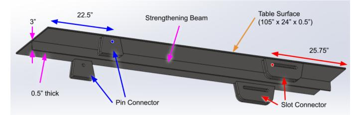
**Figure 28:** Table Surface Subsystem. Important components are labeled along some key dimensions and relations. The table has pin connectors on one end and slot connectors on the other end. Omitted from this drawing are the connection fixtures for the lockdown mechanism.
