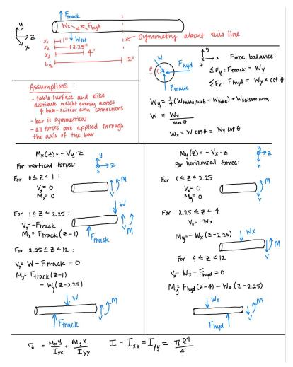
Figure 25: This figure shows the process used in the static analysis of the axle bar.
