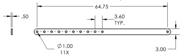
**Figure 30:** Scissor Arm Dimensions. The rightmost hole fits into the base while the leftmost hole attaches to the table surface fixtures. Note that the features defined in this drawing are not exhaustive, but rather highlight the more critical dimensions for reference.
