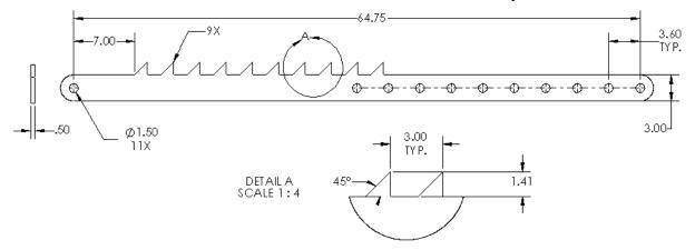
**Figure D:** Scissor Arm Dimensions. The leftmost hole fits into the base while the rightmost hole attaches to the table surface fixtures. The teeth used in conjunction with the lockout mechanism are described by Detail A. Note that the features defined in this drawing are not exhaustive, but rather highlight the more critical dimensions for reference.
