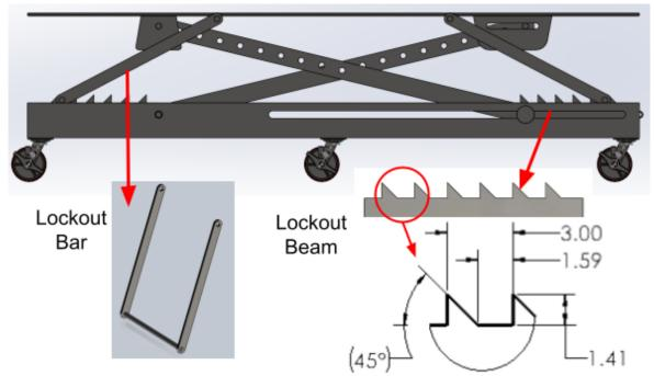
**Figure 32:** Example of lockout bars in action. As shown above, the dropdown bars rest within the notches on the base of the mechanism. The lockout bars consist of two flat stainless steel beams that are connected to each other via a round 1" plain carbon steel axle. The lockout bars are connected to the table surface at a pin fixture.
