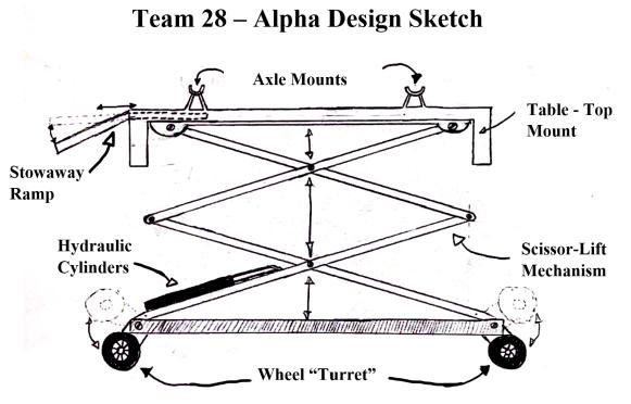
**Figure 13**: Alpha Design. Callouts depict the key features of the design. Note that dimensions are omitted as further investigation is needed to determine them. See Final Design Description below for further detail regarding dimensions and further improvements to this design.
