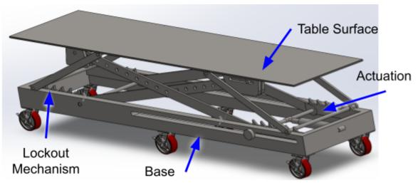
Figure 27: High level overview of final design. The main subsystems are labeled. More detailed descriptions of each can be found within their various subsections.
