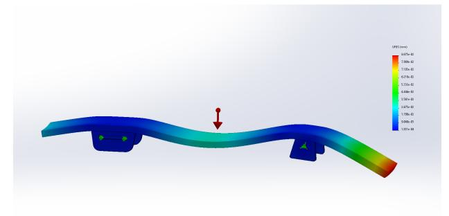
**Figure 19:** Deflection of the table surface with the Pin Axle 25 inches from the end of the table. The maximum deflection is about 0.08 mm.
