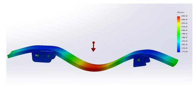
**Figure 18:** Deflection of the table surface with the Pin Axle 22.5 inches from the end of the table. The maximum deflection is about 0.04 mm.
