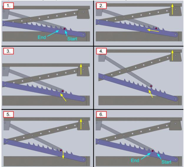
**Figure G:** Demonstrating how the lockout bar works. A section view of the mechanism is pictured with the notched scissor arm in blue while the horizontal portion of the lockout bar is pictured in red for better visibility. As the table surface is raised, the lockout bar is dragged up and over the notches. Once past the peak of the notch, the bar drops down into the notch and prevents further downward motion.
