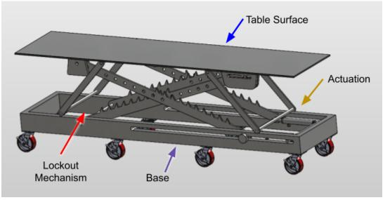
**Figure A:** High level overview of final design. The main subsystems are labeled. More detailed descriptions of each can be found within their various subsections.
