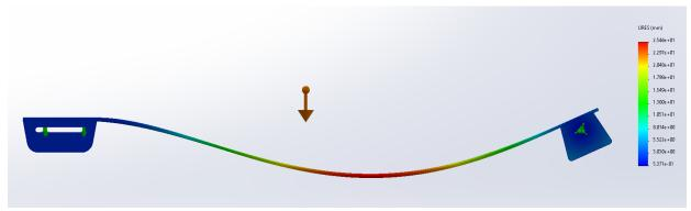
**Figure 16:** Displacement of the table surface under a distributed load of 2000 lbs. The maximum deflection is approximately 2.5 mm.
