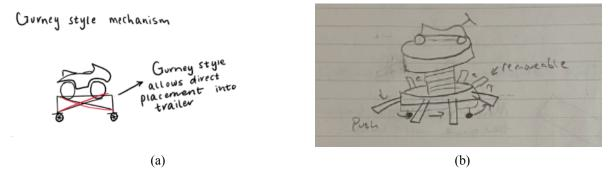
**Figure 5:** Examples of Initial Concept Generation. (a) was a quick sketch for a gurney style lift from Becca, and (b) was a rotational corkscrew style lift from Grant.
