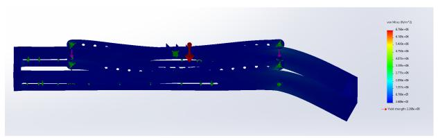
**Figure 22:** This figure shows the stresses experienced by the scissor arm and base in the low position. The maximum stress is about 6.5 MPa which is much lower than the yield stress of 220 MPa.
