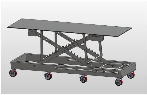
Figure F: Example of locking bars in action. As shown above, the dropdown bars rest within the notches on the scissor lift arms.
