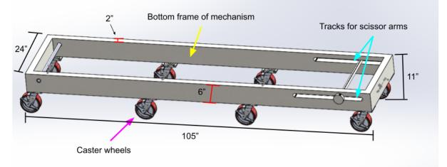
**Figure H:** Overview of Base subsystem. Important components are labeled along some key dimensions and relations. The base frame is depicted along with casters and the tracks that the scissor arms connect to.
