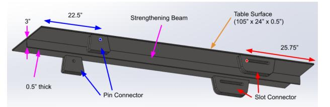
**Figure B:** Table Surface Subsystem. Important components are labeled along some key dimensions and relations. The table has pin connectors on one end and slot connectors on the other end. Omitted from this drawing are the connection fixtures for the lockdown mechanism.
