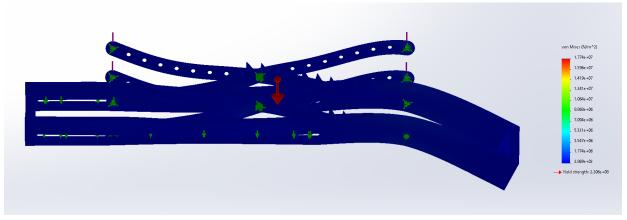
**Figure 23:** The stresses experienced by the scissor arm and base in the middle position. The maximum stress is about 12 MPa which is much lower than the yield stress of 220 MPa.
