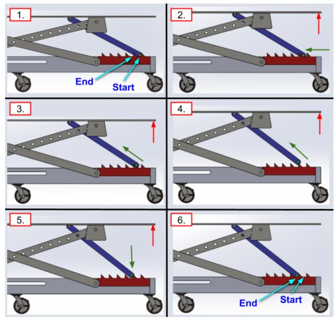
**Figure 33:** Demonstration of how the lockout bar works. A section view of the mechanism is pictured with the notched scissor arm in blue while the horizontal portion of the lockout bar is pictured in green and the lockout teeth in red for better visibility. As the table surface is raised, the lockout bar is dragged up and over the notches. Once past the peak of the notch, the bar drops down into the notch and prevents the table from moving downward.
