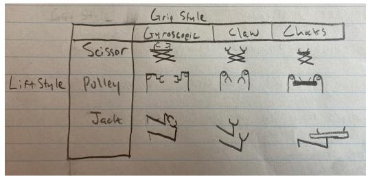
**Figure 7:** Morphological matrix variation from Grant's iteration process. The Y axis shows three design ideas for the lifting mechanism, and the X axis shows three design ideas for the bike grip style. In total, 9 unique and quick ideas were created from this process.
