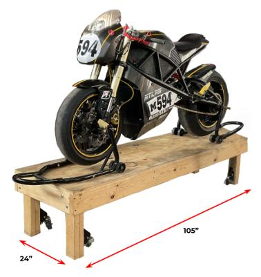
**Figure 1:** SPARK's Current Motorcycle Setup. Pictured is their current project, ATLAS, on the wood platform held in place by purchased Venom chock stands. Not pictured is the overhead winch used to lift the motorcycle from floor level onto the platform. The dimensions of the platform are shown by the red arrowheads.
