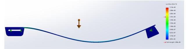
**Figure 15:** Stresses experienced by the table surface under a distributed load of 2000 lbs. The maximum stress is about 311.6 MPa, which is greater than the yield stress. Therefore, the table surface would yield under these conditions.
