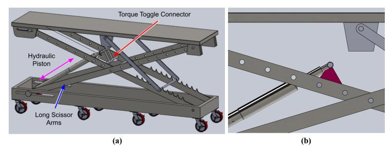
**Figure 31:** Previous actuation designs. (a) depicts the previous version of the assembly. Some features of note are the longer scissor arms, the wider scissor arm connection fixtures on the table surface, the angled hydraulic piston, and the torque toggle connector. (b) depicts the now obsolete torque toggle connector, highlighted in red for visibility.
