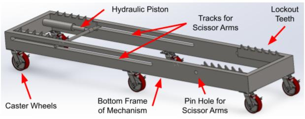
Figure 34: Overview of Base subsystem. Important components are labeled along some key dimensions and relations. The base frame is depicted along with casters and the tracks that the scissor arms connect to.
