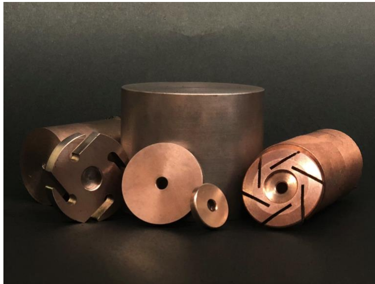
Figure 6.1 CuCr and CuCrW contact materials produced using developed pressure-less infiltration method
