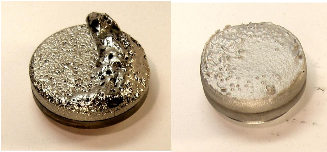
Figure 4.1 Excessive arc-erosion on VAPD targets due insufficient thermal conduction as a result of high porosity
