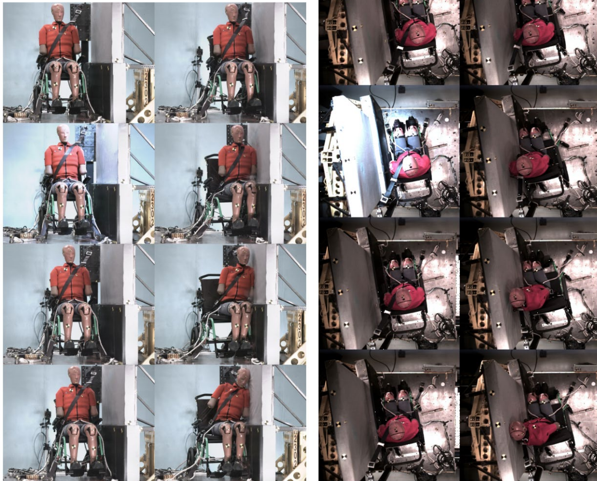
Figure 133. Kinematics for WX2302, Leggero+SWTORS, nearside with wall, from -20 to 120 ms every 20 ms.
