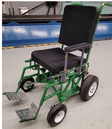
Figure 76. Photo of the SWCSI, modified from the SWCB to includes different wheels and attachment bolts, a shifted lap belt anchor location, a left armrest, and a contoured seat cushion.
