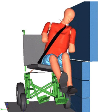
Figure 58. Peak excursion comparison of FE model of SWCB secured by SWTORS to test WX2207 under nearside impact.
