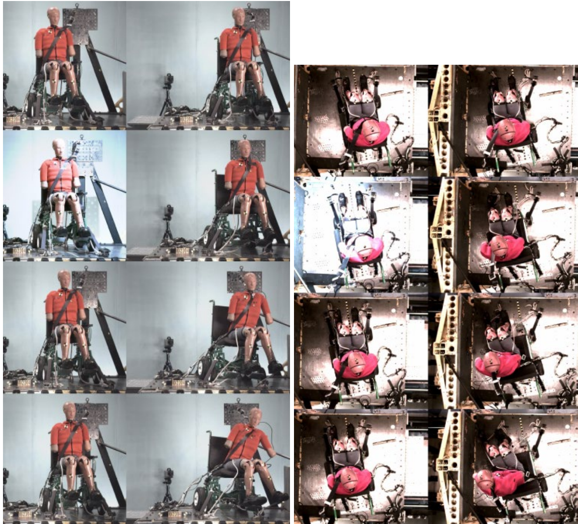
Figure 141. Kinematics for WX2304, SWCSI+SWTORS, nearside (center) without wall, from -20 to 120 ms every 20 ms.
