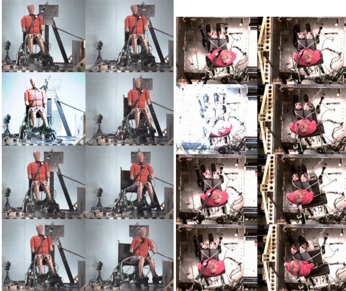
Figure 140. Kinematics for WX2310, SWCB+SWTORS, nearside (center) without wall, from -20 to 120 ms every 20 ms.
