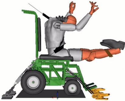
Figure 93. Comparison of model and test kinematics for SWCB with detailed SWTORS, under frontal impact, at ~ 30, 60, 90, 120 ms.
