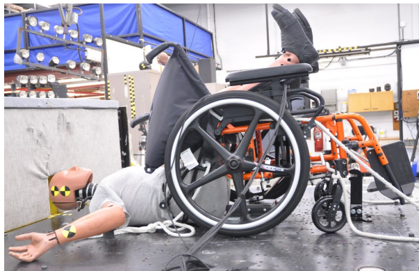
Figure 28. Back support attachment hardware also failed, allowing ATD to fall out of chair.
