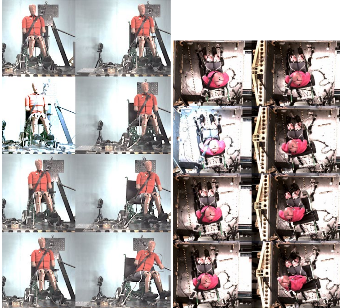
Figure 142. Kinematics for WX2306, SWCSI+SWTORS, nearside (center) without wall, from -20 to 120 ms every 20 ms.
