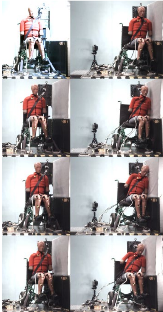
Figure 136. Kinematics for WX2303, SWCSI+SWTORS, nearside with wall, from 0 to 140 ms every 20 ms.
