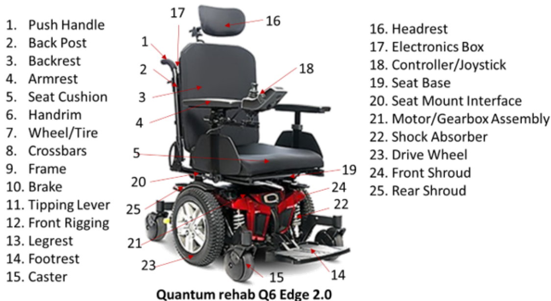
Figure 104. Photo of power wheelchair and labeled components.
