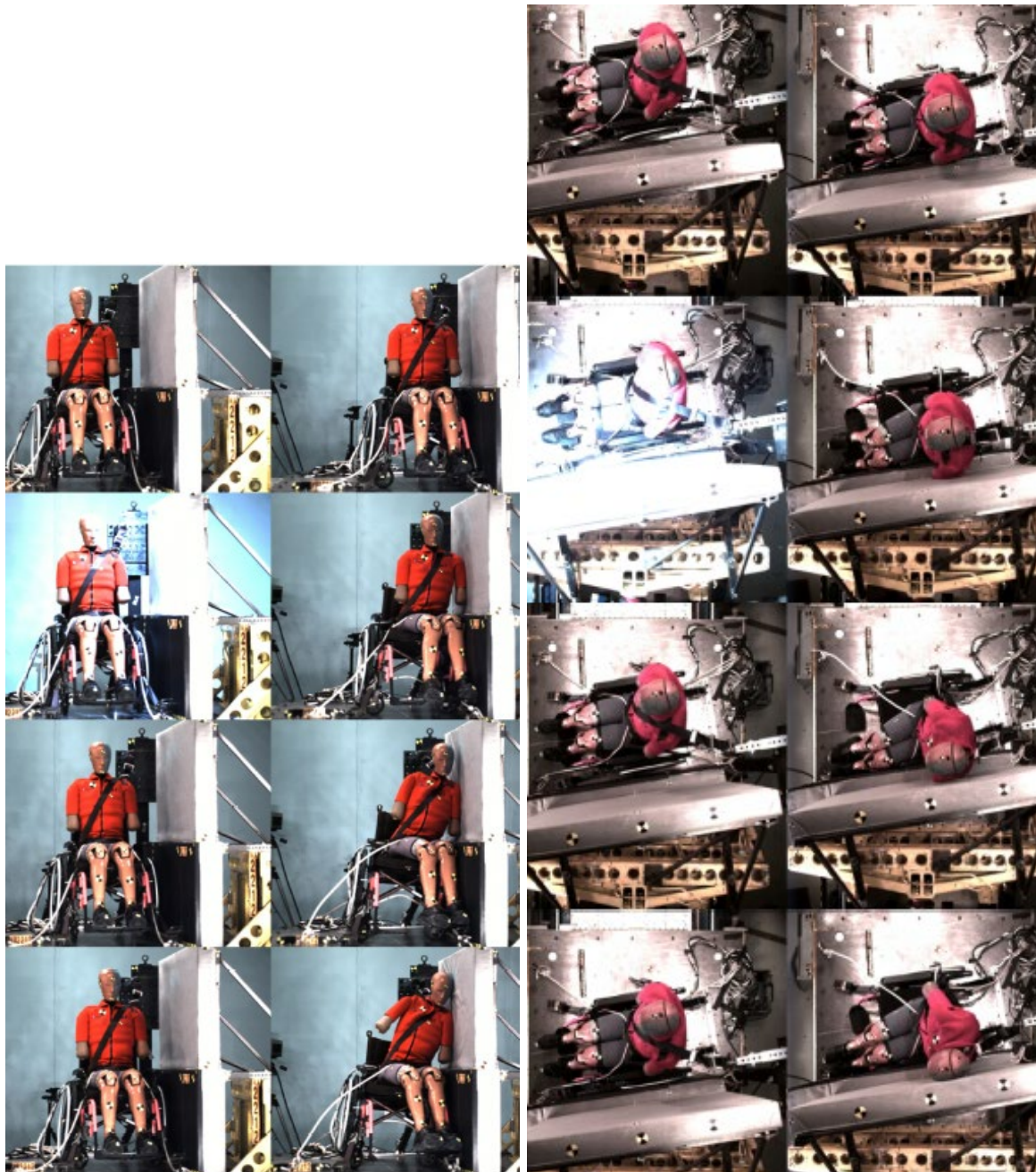
Figure 131. Kinematics for WX2212, Ki Mobility+SWTORS, nearside with wall, from -20 to 120 ms every 20 ms.
