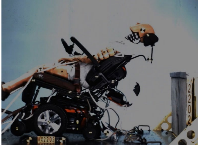
Figure 29. Peak rearward movement of ATD in power wheelchair secured by commercial 4-point strap tiedowns.
