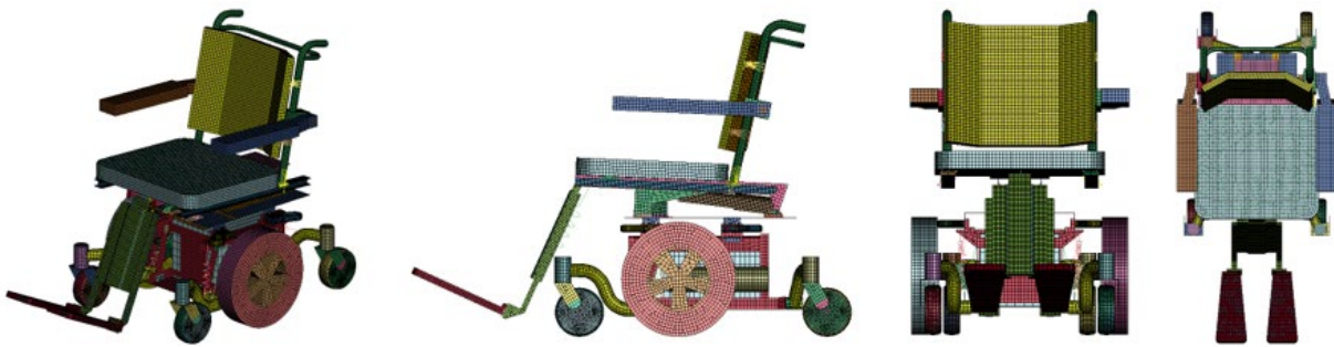
Figure 105. CAD geometry used to create power wheelchair model.
