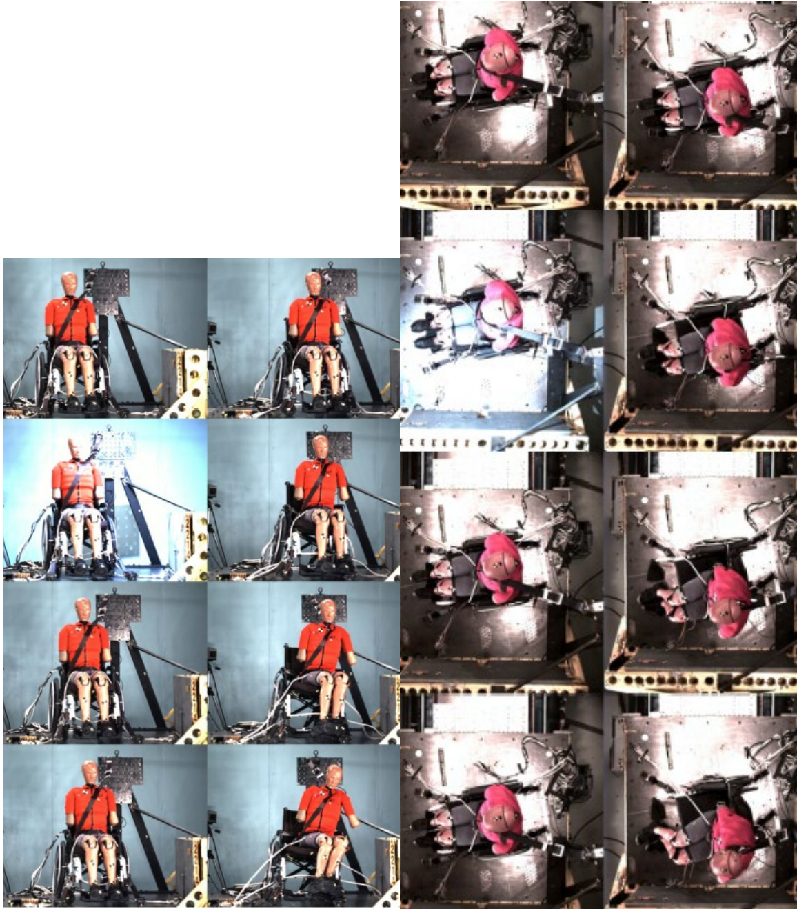
Figure 138. Kinematics for WX2214, Quickie 2+SWTORS, nearside (center) without wall, from -20 to 120 ms every 20 ms.
