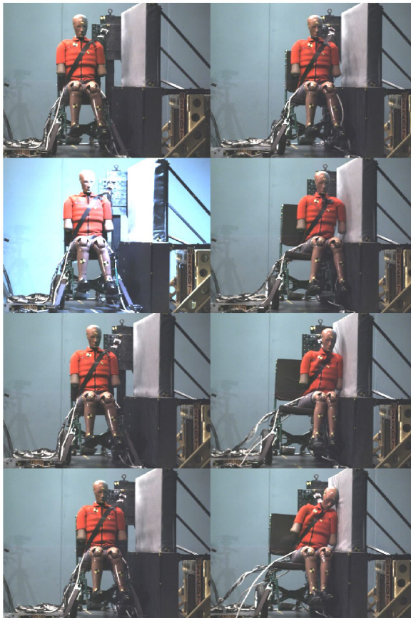
Figure 135. Kinematics for WX2207, SWCB+SWTORS, nearside with wall, from -20 to 120 ms every 20 ms.
