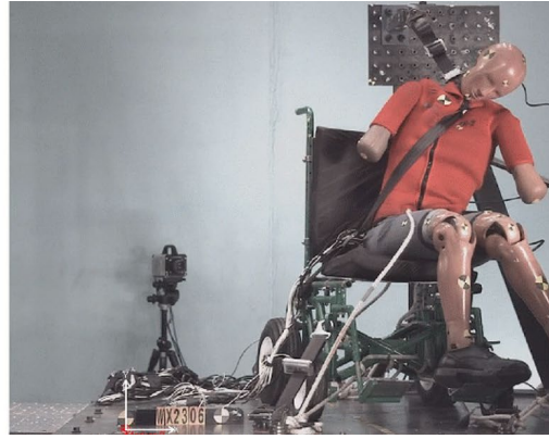
Figure 59. Peak excursion comparison of FE model of SWCSI secured by SWTORS to test WX2306 under nearside (center) impact.
