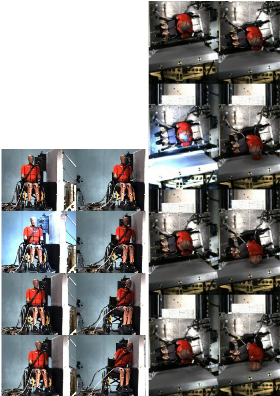
Figure 132. Kinematics for WX2208, Quickie 2+SWTORS, nearside with wall, from -20 to 120 ms every 20 ms.
