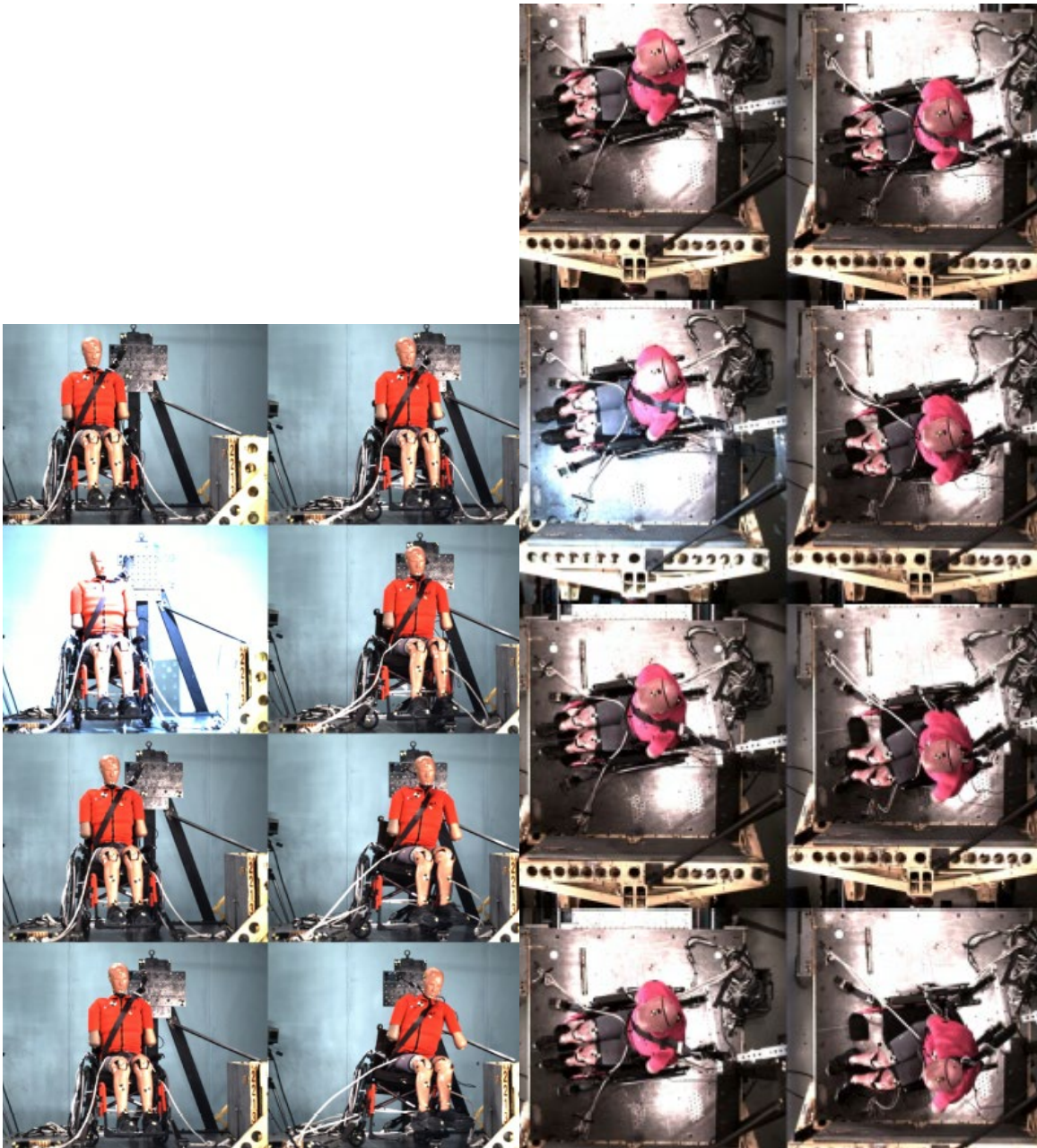
Figure 137. Kinematics for WX2213, Ki Mobility+SWTORS, nearside (center) without wall, from -20 to 120 ms every 20 ms.
