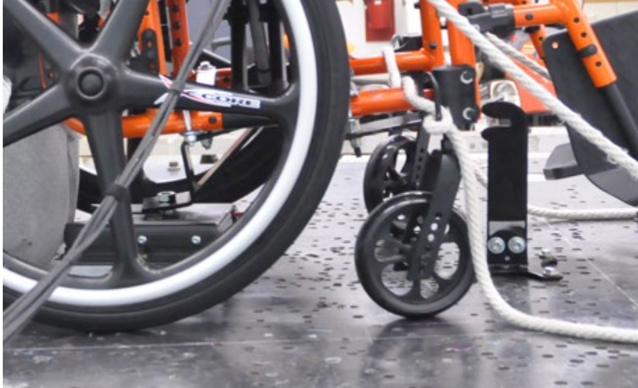
Figure 27. Wheelchair disengaged from front stabilization hook, leading to deformation of main mounting bracket.
