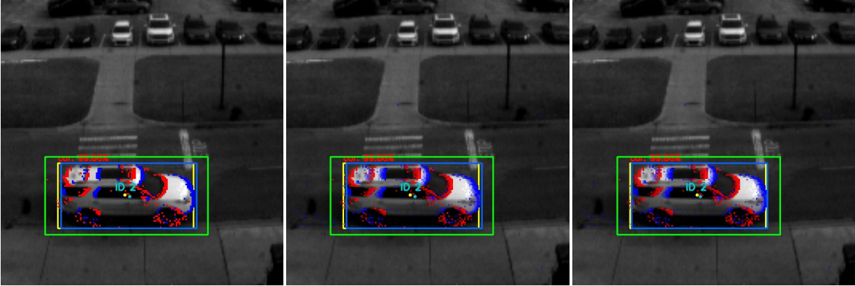
(a) Event-based mask with a discrete-step moving window. (b) Event-based mask with a temporally-weighted moving window. (c) Edge-based mask with a temporally-weighted moving window.
