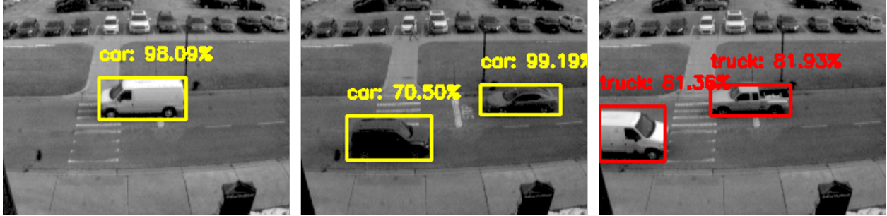
Figure 3.2: Object detection output on sample images for one of the scenes in our dataset. The object detector used in this figure is YOLOv3 [149]. In this scene, static objects, such as the parked vehicles in the top half of the scene, are disregarded.
