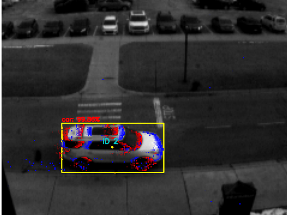
Figure 3.8: Demonstration of an image with temporally weighted events (visualized by the transparency effect) overlaid on top. Faded blue and red dots resemble older positive and negative events, respectively. This scene represents the same time instance as the one shown in Figure 3.4 at a tracking rate of 48 Hz, though with an extended 50 ms of event data history compared to 21 ms.
