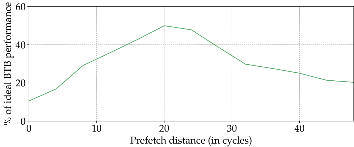
Figure 6.26: Twig’s average performance variation in response to increasing the prefetch distance. Across different applications, Twig provides greatest benefit with prefetch distance 15-25 cycles.
