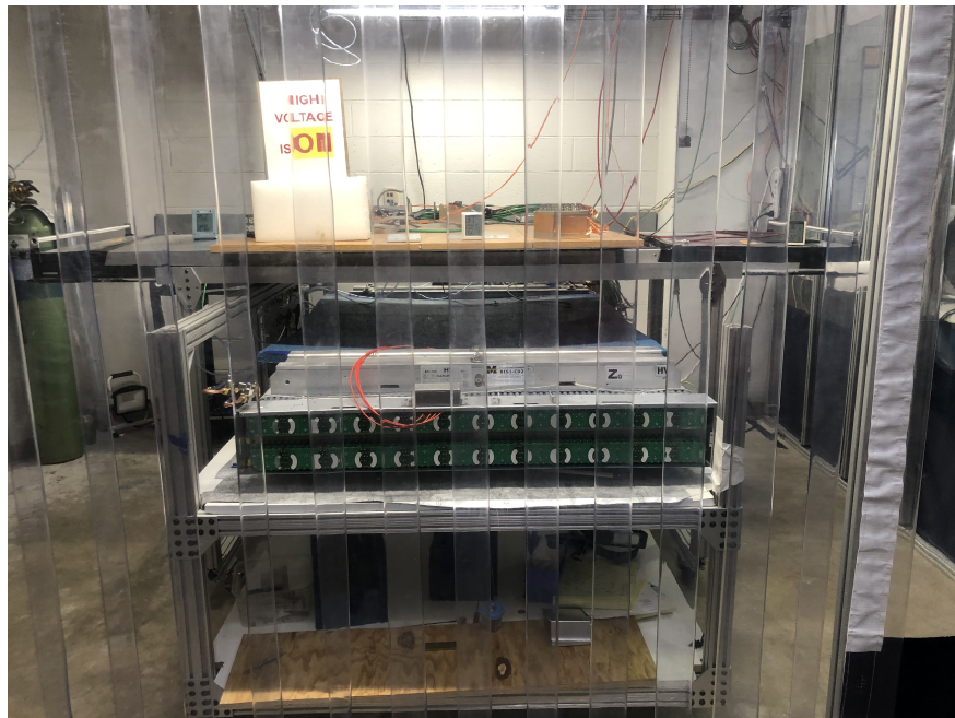
Figure 3.14: sMDT cosmic ray test station in a humidity-controlled room. The sMDT chamber sits on a cart with a 1.5m 2 scintillator mounted above. In this image the Faraday cage is not yet fully assembled and the HV HH cards are seen on the chamber.
