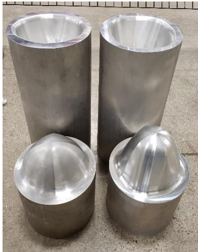
Figure D3: The profiled-billet pairs extruded during the 2021 rectangular bar study.
