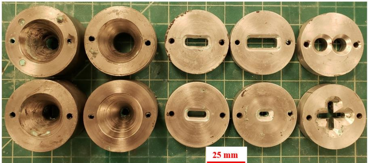
Figure 4.3: From left to right: Axisymmetric die set; rectangular die set; complex dies with dual-circle die on top, cross die on bottom.
