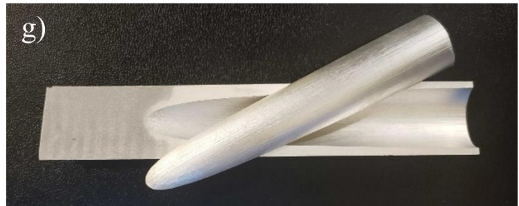
Figure 3.17: Shear test fracture morphology. The samples were extracted from the AA6061 round bar, single-piece billet extrusion, with butt shear (except where specified otherwise).
