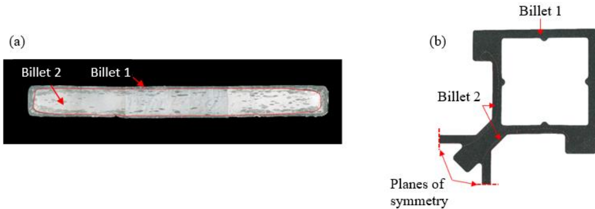
Figure A1: Example cross sections of case study profiles (a) rectangular solid (70% billet 2 area) and (b) 80-20 T-slot bar (23% billet 2 area) used to measure the transverse weld length.
