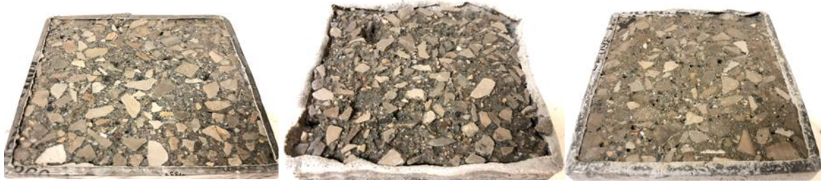
Figure 4.6 Surface of 039-4%SF exposed to pure water (left), 3% salt solution(middle), and 12% salt solution (right)
