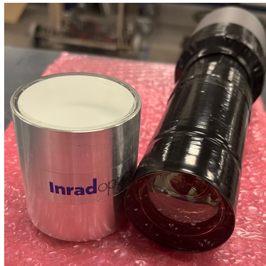
Figure 2.11. Photograph of the 5.08 cm in length and 5.08 cm in diameter trans -stilbene crystal and a 5.08 cm in diameter photomultiplier tube.
