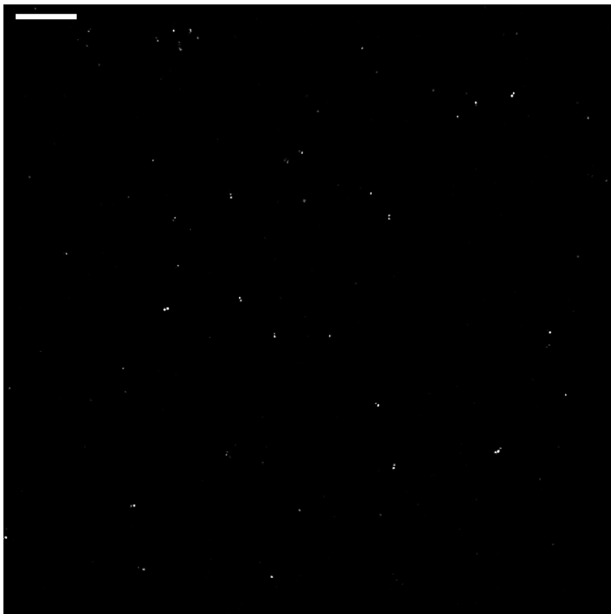
Supplemental Figure 5.14 10 \mu\text{m} by 10 \mu\text{m} region showing DNA origami rulers analyzed in Figure 5.3. The full imaged area was 40 \mu\text{m} by 40 \mu\text{m} . Scale bar is 1 \mu\text{m} .
