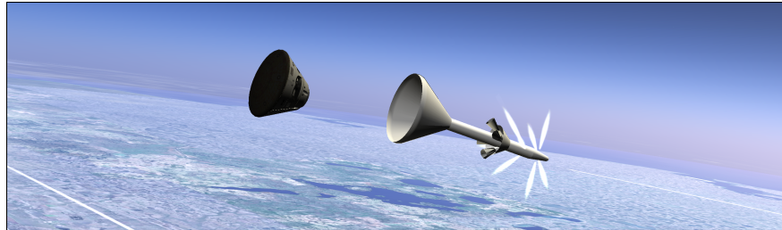
Figure 2.8: IGOR Spaceflight Simulation — Orion AA-2 simulation moments after the crew module (left) separates from the launch abort system (right).
