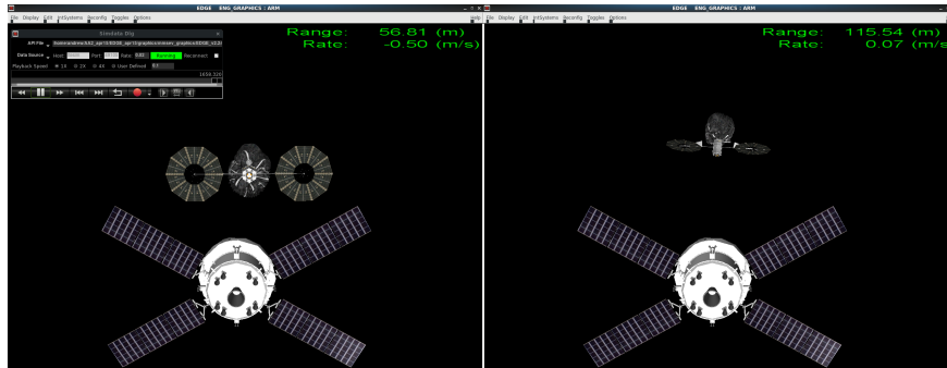
Figure 4.11: Asteroid Redirect Mission — NASA spaceflight simulation without (left) and with (right) PCSPOOF. PCSPOOF caused a significant deviation in the vehicle’s flight path, which prevented docking.
