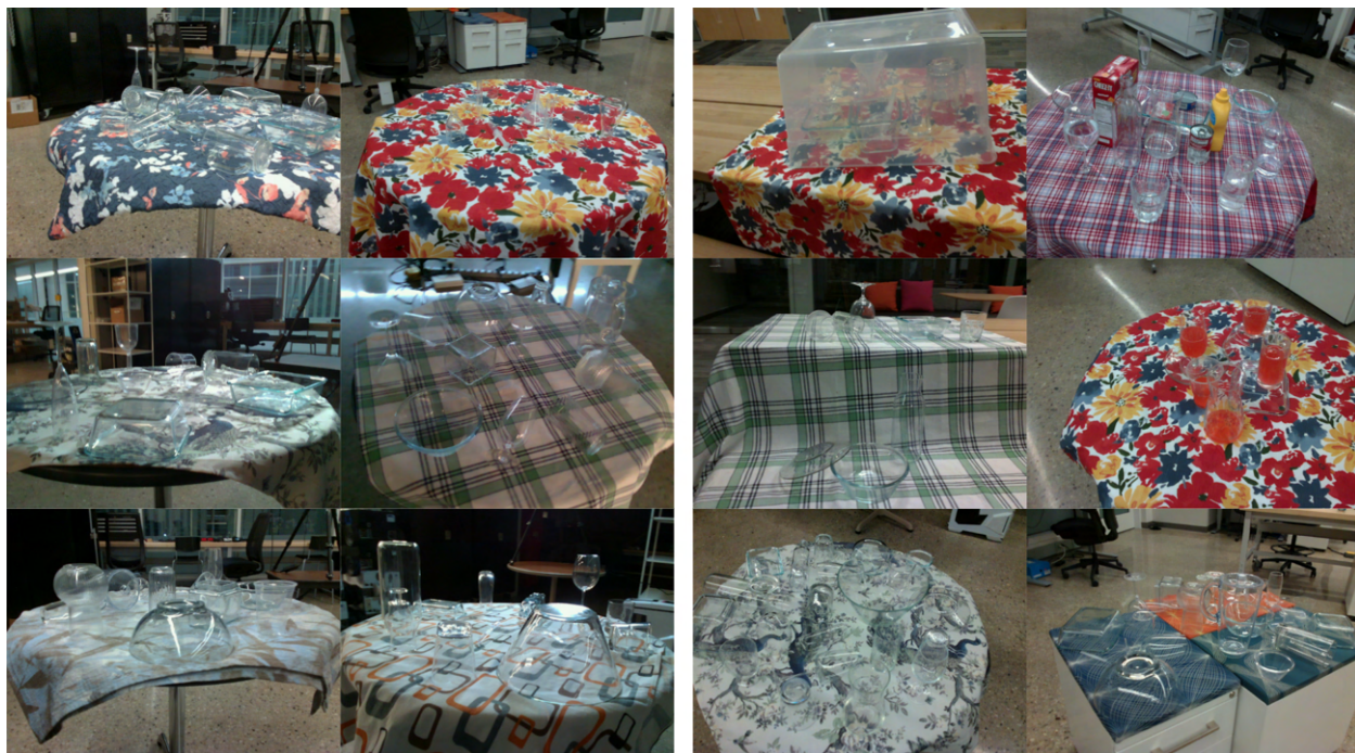
Figure 6.2: Sample images from ClearPose dataset. On the left, we show RGB images taken for different object subsets under various lighting conditions and backgrounds. On the right, we show examples of different types of testing scenes, such as covered by a translucent box (top-left), novel background with opaque distractor objects (top-right), non-planar cases (middle-left), filled with liquid (middle-right), and heavy clutters of transparent objects (bottom).
