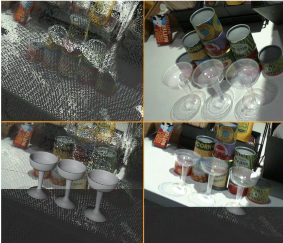
Figure 5.9: The labelling on transparent champagne cups. When there is no reliable depth (top-left), ProgressLabeller enables checking the pose validity by re-projection object models (bottom-left) to RGB images from different views (top-right and bottom-right).
