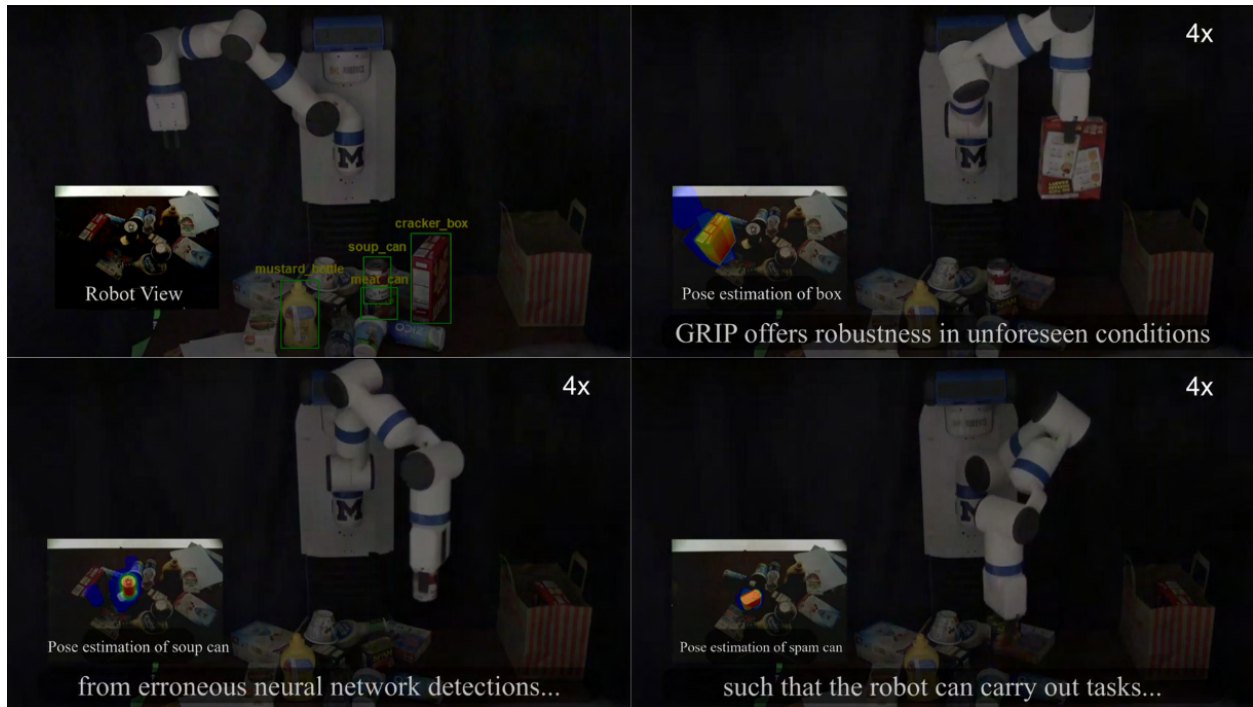
Figure 3.8: A Fetch robot is packing grocery based on pose estimates from the GRIP pipeline.
