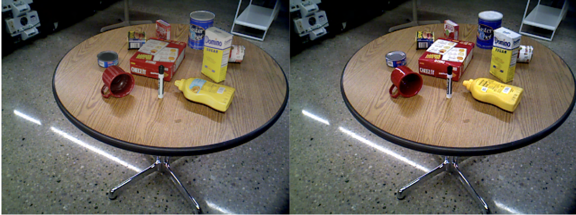
Figure 5.6: A synthesized RGB image using Blenderproc is shown on the left. The original image is shown on the right. The YCB objects are rendered and overlaid to original image according to labelled poses. Depth synthesized images are generated in the same way.
