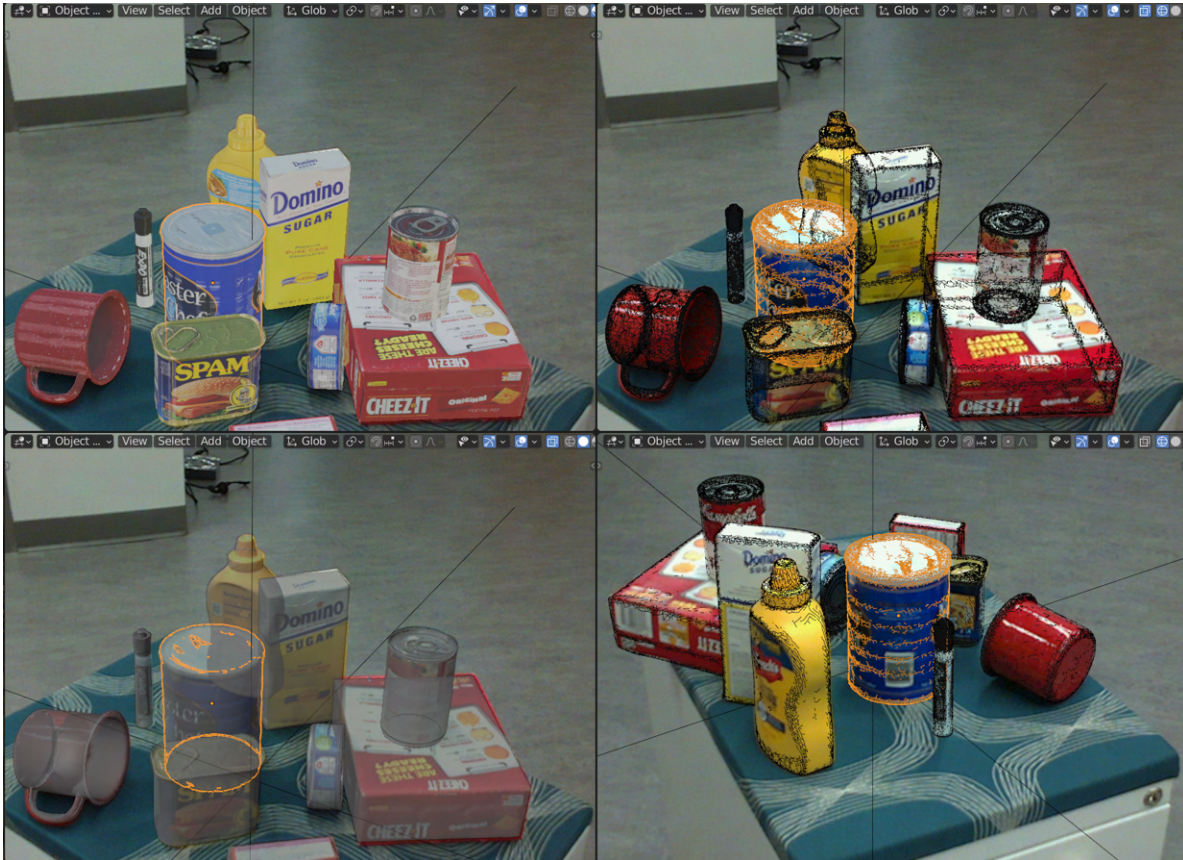
Figure 5.2: Capture of ProgressLabeller user interface for multi-view re-projection checking. The top-left view shows the aligned object models with rendered texture at labelled poses. The bottom-left view and top-right view show the silhouettes and boundaries respectively at the same camera view, and the bottom-right view shows the boundaries from another view for validation.
