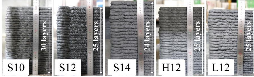
Figure 4.7: Side views of the printed box elements.
