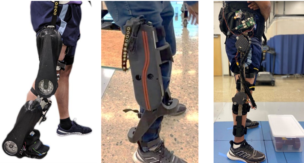
Figure 1.1: Improvements in exoskeleton hardware. Left: Comex1 second generation knee ankle exoskeleton. Middle: Comex2 second generation knee only exoskeleton. Right: M-Blue modular hip-knee, hip only, and knee only exoskeleton (hip-knee configuration shown).
