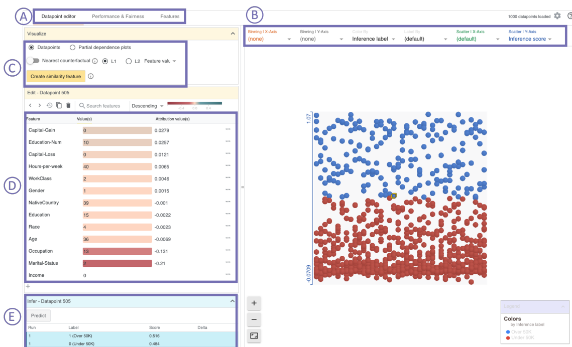
Figure 4.4: The landing interface of Google’s What-if Tool showing the Datapoint Editor. Users can access different tabs related to the data, model performance, and features (A). Each tab has its own interactive elements with similar density of features as the Datapoint Editor. The scatter plot representing the data can be updated based on several options, such as binning x and y axes and scattering data using different labels (B). Users can also compute additional information about the datapoint, such as counterfactuals, local partial dependence plots, comparison with the same datapoint’s prediction from a different model (C). Individual input feature values are editable for interactive what-if testing, for the selected datapoint on the scatter plot (D). In this case, I set up the tool to also provide SHAP attribution values as local explanations (D). The inference section for the selected datapoint (E) allows users to get real-time predictions for any edited input features from (D).
