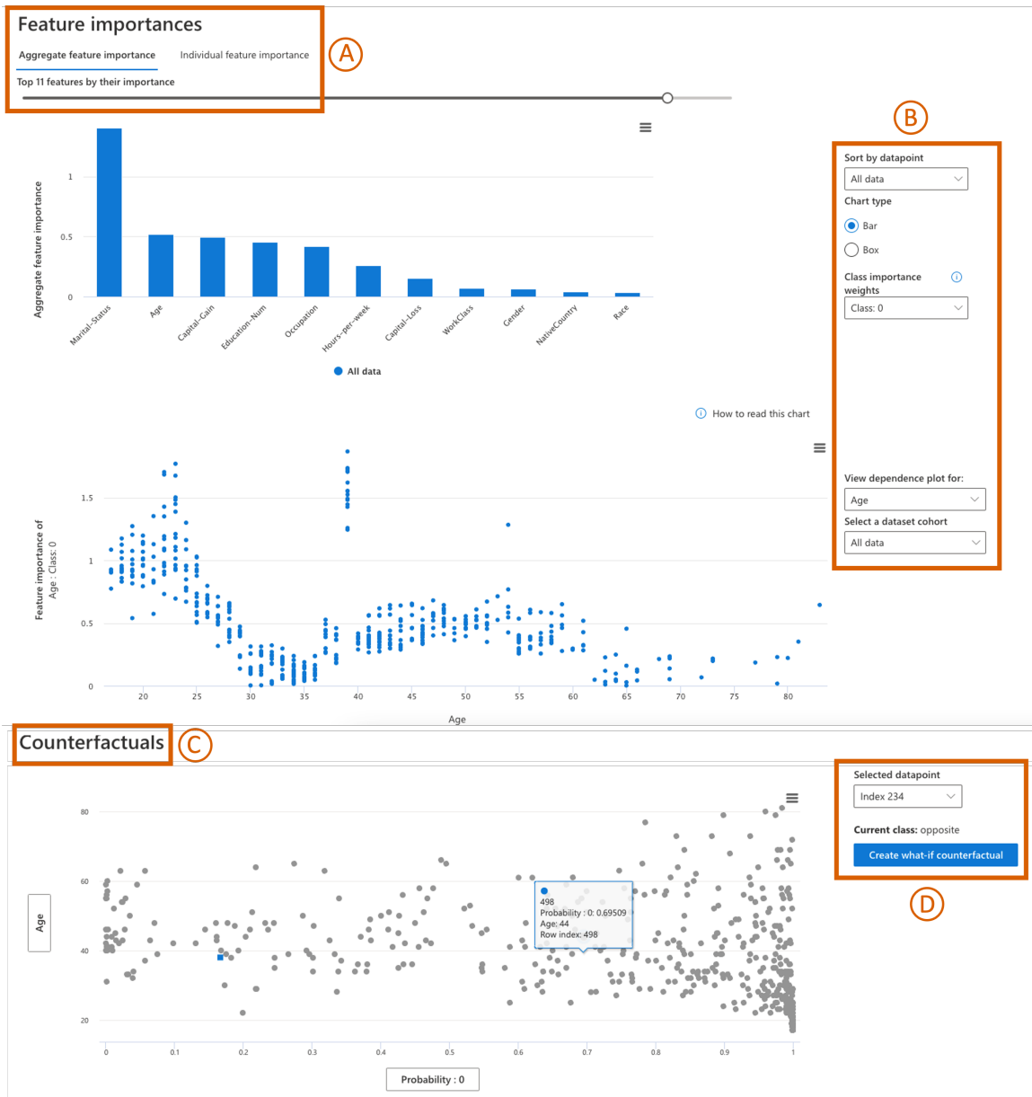
Figure 4.3: The landing interface of Microsoft’s Explanation Dashboard with minor edits to reduce whitespace. The dashboard includes several exploration sections. Here I show two of them, for Feature Importances (A) and Counterfactuals (C). Each section has its own set of interactive visuals and controls. Users can view aggregate or individual feature importances, and clicking on a feature bar shows the partial dependence plot (the middle one here). There are several sorting and binning options for displaying this data (B). The counterfactuals section allows users to select datapoints, view their local explanations (not shown here), and create what-if counterfactuals (D) which opens a new pane with various editing and sorting options for the suggested counterfactuals.
