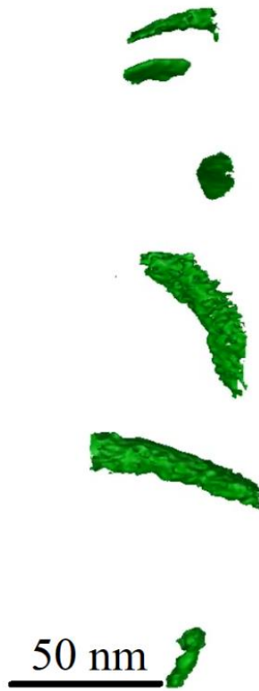
Figure B 8: Solute-decorated dislocation loops (using 50 at. % Ni isosurfaces) in Cr 0.5 FeNi at 10 dpa using 10 -4 dpa/s at 500 °C.
