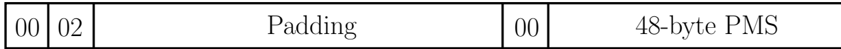
Figure 5.4: PKCS#1v1.5 RSA encryption padding. It appends a pseudorandom padding string to the message, together with some fixed bytes. The padding block is filled with k - 3 - \ell non-zero bytes that are generated by a pseudorandom number generator, where k is the byte-length of the modulus and \ell is the byte-length of the message to be encrypted.
