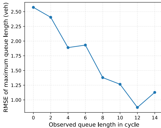
Figure 4.18: RMSE of the maximum queue length estimation with different observed queue lengths (for all those cycles with only one observed trajectory).
