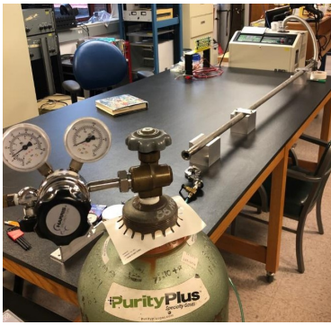
(a) Gas tightness test station. (b) Interior side of tube. (c) Vacuum side of tube.
