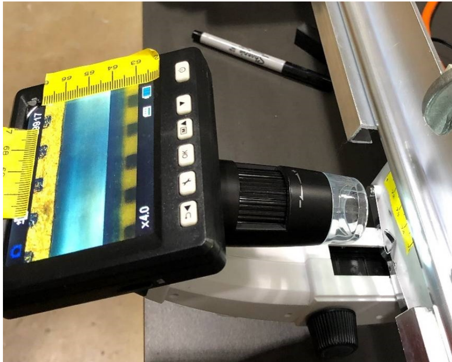
Figure A.4: Tube straightness measurement station with the digital microscope aimed at the middle of the aluminum tube sitting on the V-bar.
