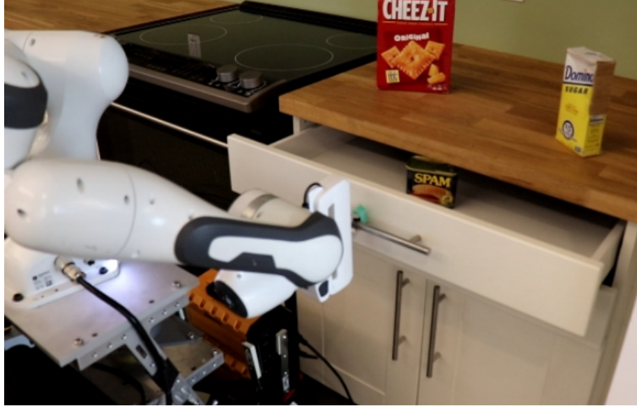
Figure 2.2: The robot pulls open a drawer to detect whether the spam object is at a continuous pose particle within the drawer. Figure adapted from Garrett et. al. [37]
