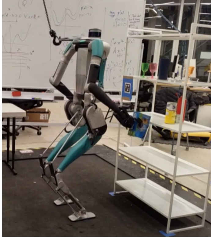
Figure 1.2: The Agility Robotics Digit Bipedal Humanoid Robot stocking a shelf with a cookie box. Figure adapted from Adu-Bredu et. al. [2]
