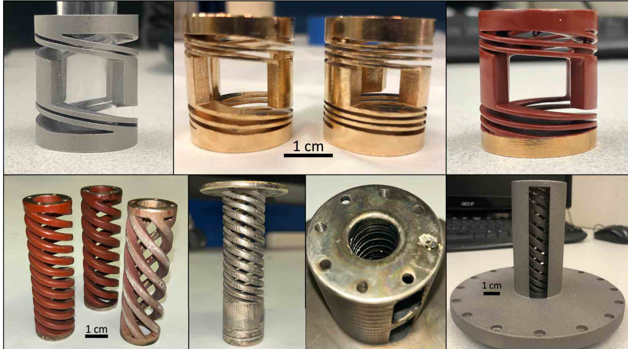
Figure 3.2: Various helical load hardware designs for MAIZE, showing the flexibility afforded by 3D-printing. Printing methods include binder-jet (steel 316/bronze alloy), DMLS (steel 316), and lost-wax casting (bronze or brass). Red parts are coated in a dielectric paint called Glyptal.
