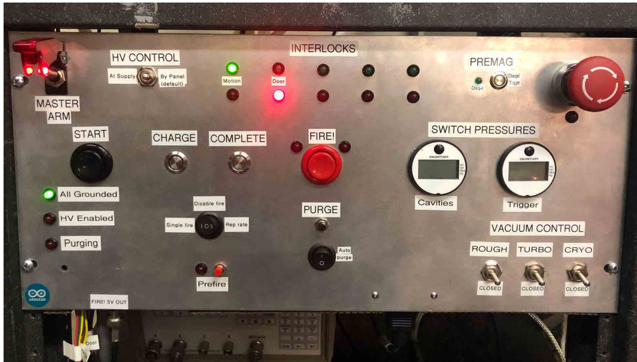
Figure C.4: Arduino Uno (ATmega328P-based) control panel for semi-autonomous control of the BLUE charging and firing sequence, as well as other system functions.
