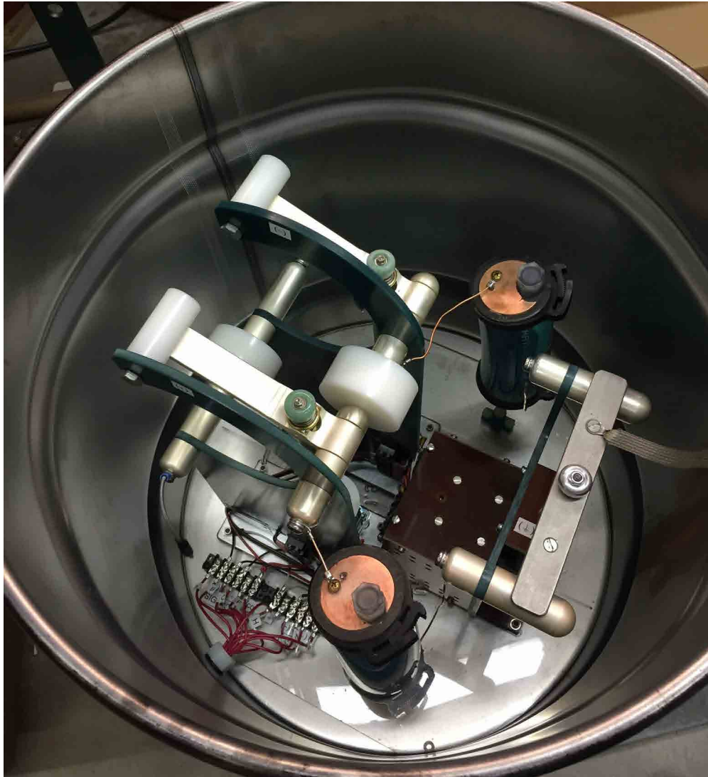
Figure C.5: A 20-gallon oil drum contains the three Ross HV relays used in the charging circuit. The relays are operated by the control panel (see Sec. C.3.1 and Fig. C.4) during the charging sequence. The large copper-sulfate dump resistors in this photograph were ultimately replaced with 50-k \Omega ceramic resistors.
