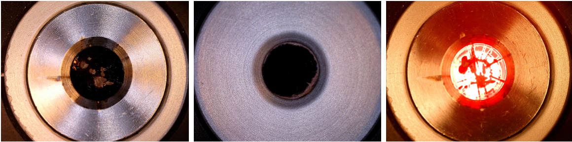
Figure A.9: Microscopic images of the GaSe crystal damaged in the OPCPA experiment. (a) Front surface (incident surface). (b) Back surface. (c) Bulk of the crystal by illuminating from the back.
