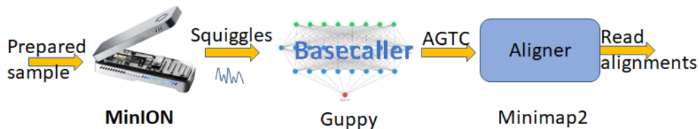
Figure 1.3: A basic MinION sequencing pipeline
