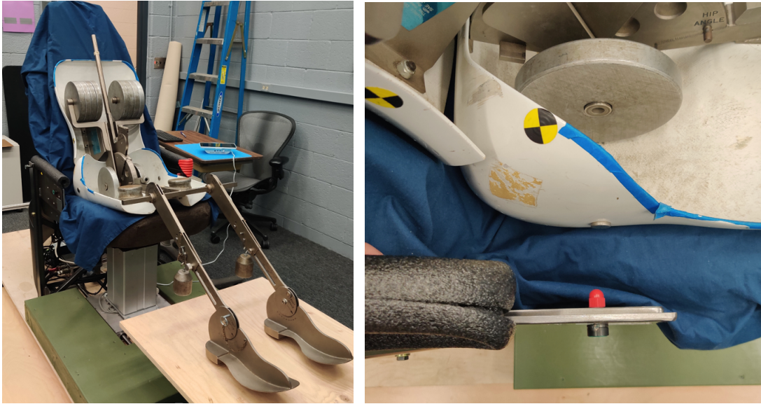
Figure 2. SAE J826 H-point machine and the H-point alignment with the seat back pivot.
