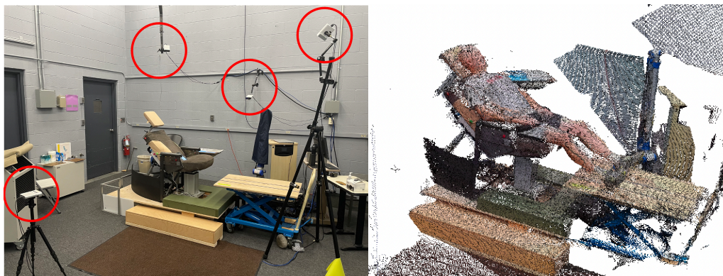
Figure 6. Location of cameras used for posture measurement and an example 3D point cloud.
