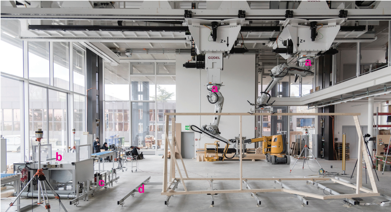
2 ETH Zurich's Robotic Fabrication Laboratory (RFL): a) industrial robotic arms attached to a gantry system; b) CNC saw; c) end-effector docking station; d) assembly stand.
