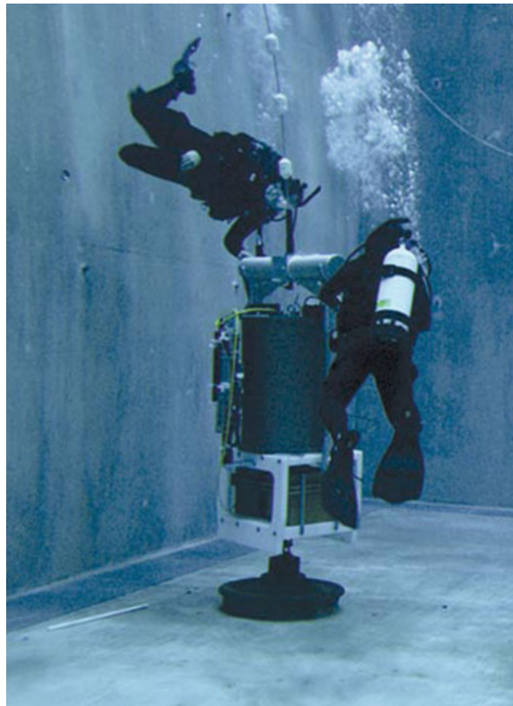
Fig. 2. The second-generation Environmental Sample Processor (2 G ESP) being tested in a seawater tank ahead of deployment in Monterey Bay. The instrument is moored subsurface and an electromechanical cable provides for communications between a remote station and the ESP's surface buoy. An integral conductivity-temperature depth (CTD) package is visible at left. The ESP operates on 12-V rechargeable batteries (at bottom, above the anchor). Photo credit: Todd Walsh, Monterey Bay Aquarium Research Institute (19).
