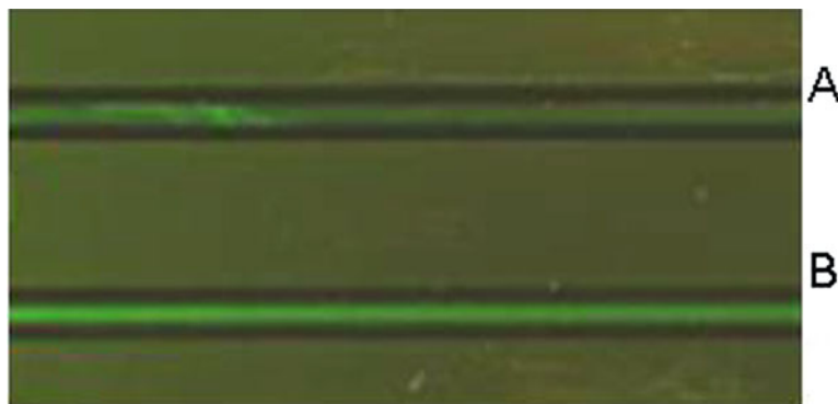
Fig. 9. Visualization of probe attachment inside capillaries, silanized after baking (a) or ozone treatment (b). Capillaries were coated with Cy3-labeled capture probe (Amn-Vibcap-Cy3) and were visualized using a microarray scanner and a slotted polycarbonate holder.
