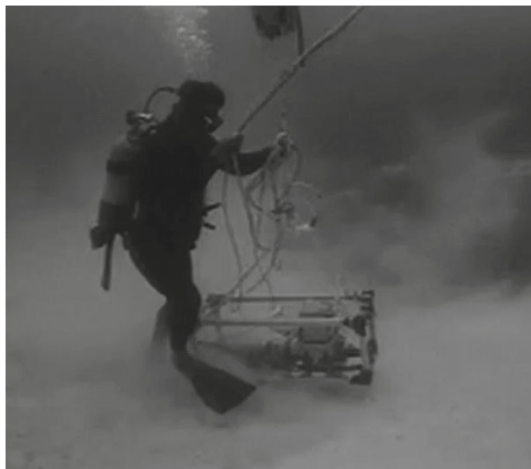
Fig. 9. IISA-ATP deployed by diver at submarine hydrothermal site at coral reef off Taketomi Island.
