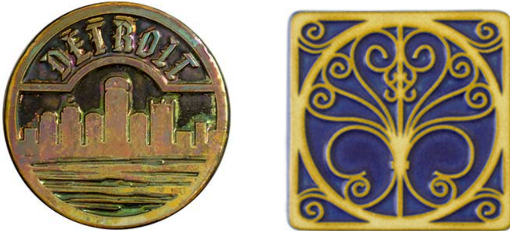
Figure 1. Tile iridescence varies by firing and glazing process. Iridescent tile at left. Non-iridescent tile at right. Images courtesy of Pewabic.
