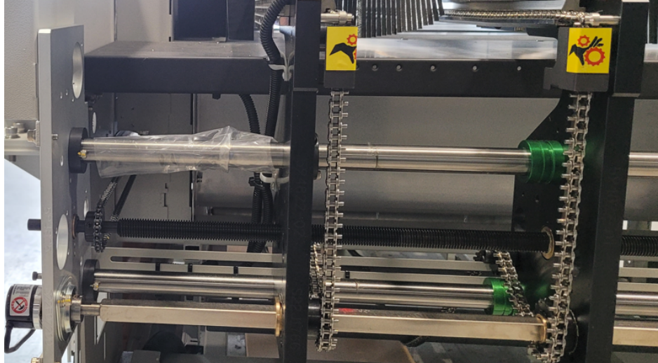
Figure 4: Right side of Heller Industries reflow oven with side panels removed. Sprocket on the left side near the aluminum plate is connected with a chain to the width adjustment chain sprocket shown in Figure 3. The chain ensures all lead screws (and edge hold rails) move synchronously.
