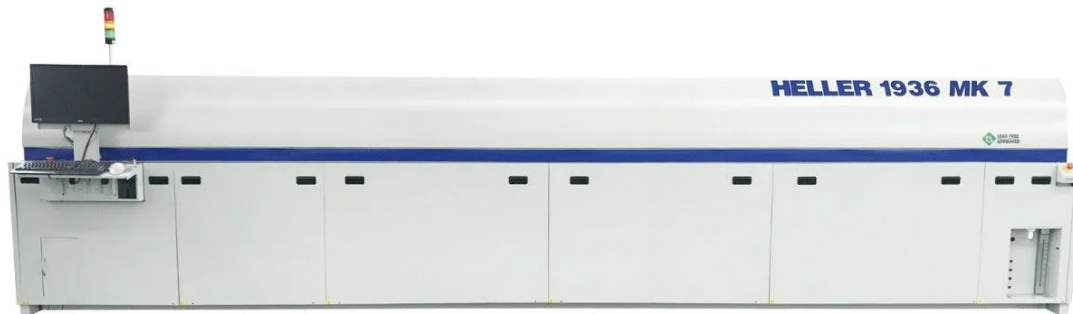
Figure 1: Heller Industries 1936 MK7 reflow convection oven with the top closed. Reflow convection oven refers to the oven being heated by the recirculation of nitrogen inside the oven [5].
