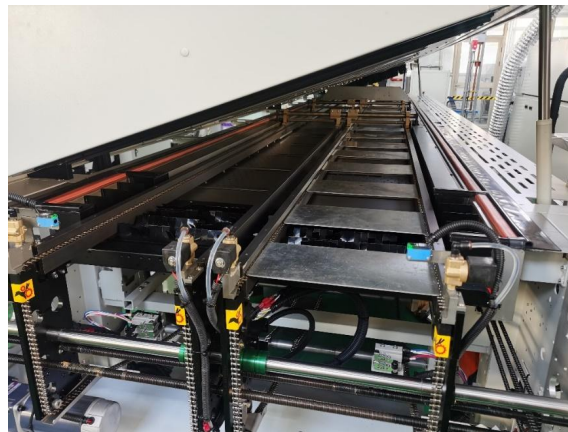
Figure 2: View of EHC system in Heller reflow oven, with top open. This view is from the entry of the oven. Placeholder boards are lined up along the right lane to demonstrate the edge hold capability. This specific model features dual lanes to double output.
