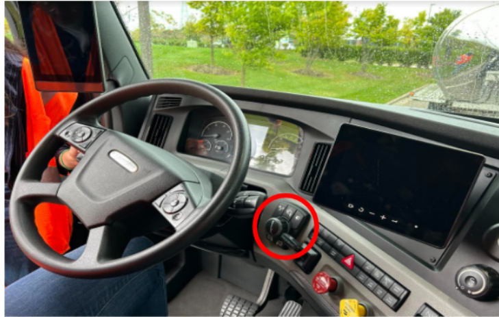
Figure 11: Location of the MirrorEye CMS controller (circled in red) inside the truck cab
