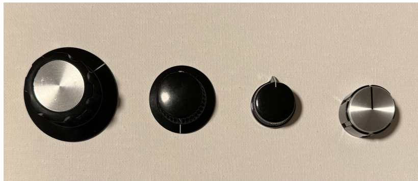
Figure 21: Four knobs used for testing ergonomics for users for the rotary knob. Dial One starts from the left to Dial Four on the far right
