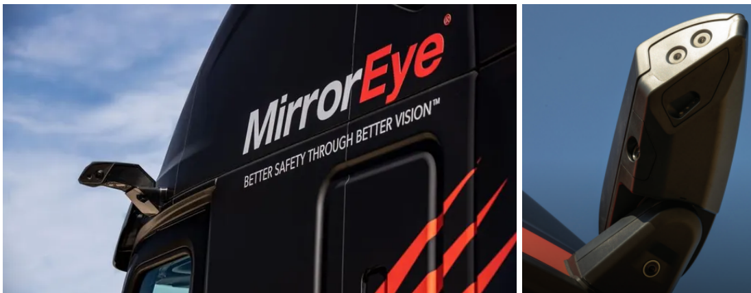
Figure 1: A total of 5 external Mirror Eye cameras including 2 on the driver's side wing (left) mounted above the cab door and 3 on the passenger side wing (right)
