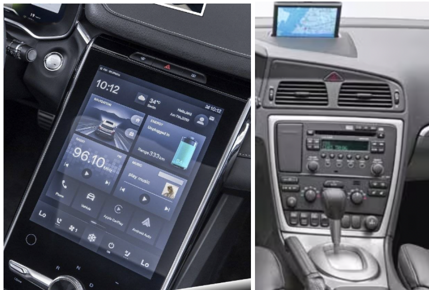
Figure 10: Examples of HMI systems used in Vi Bilagare’s case study. Left: Chinese electric car, MG Marvel R’s HMI system. Right: 2005 Volvo V70’s HMI system.
