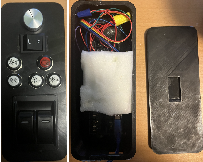
Figure 19: 3D printed iteration one build module front(left) and inside housing unit with lid(right)
