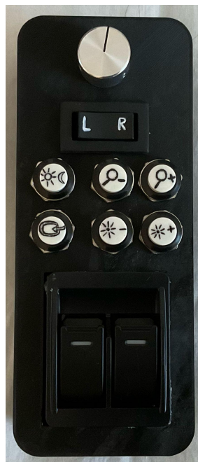
Figure 24: Final Module 3D printed with a rotary knob, rocker switch, six buttons, and window switches
