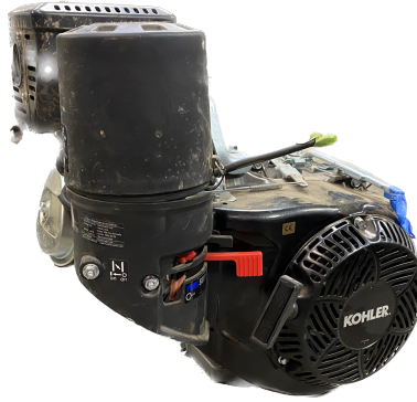
Figure 2.3.2. A Kohler gasoline engine Command Pro Small Horizontal series CH440 Model. This is the engine that SAE specifies Baja Racing Teams must use.
