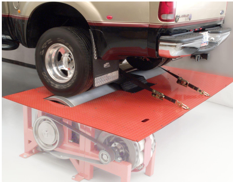
Figure 3.1.2. An automotive-sized chassis dyno [10].
