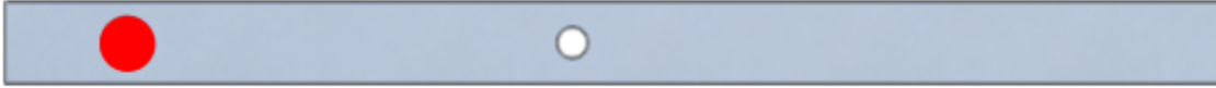
Figure D29: The mounting hole for the 1/2" bushing on stiffener B, marked in red.
