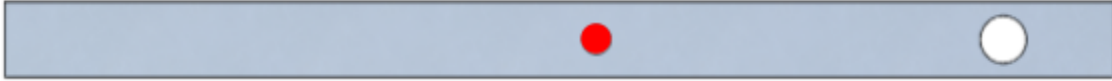
Figure D23: The mounting hole for the 1/4" bushing on stiffener A, marked in red.
