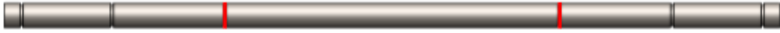
Figure D33: The mounting grooves for the 1/4" retaining rings on the ramp shaft, marked in red.
