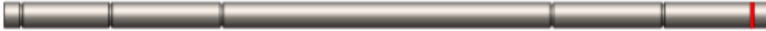
Figure D57: The mounting groove for the 1/4" retaining ring on the ramp shaft, marked in red.
