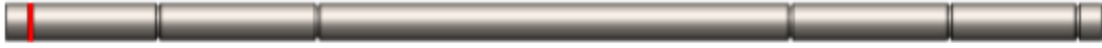
Figure D69: The mounting groove for the 1/4" retaining ring on the ramp shaft, marked in red.
