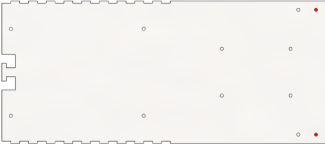
Figure D7: The mounting holes for the front bracket on the base plate, marked in red.
