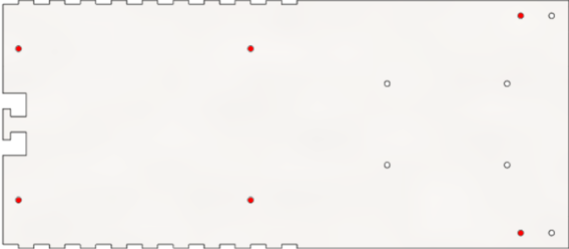
Figure D5: The mounting holes for the bumpers on the base plate, marked in red.
