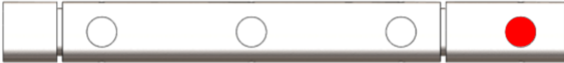
Figure D51: The mounting hole for the release handle on the release master, marked in red.
