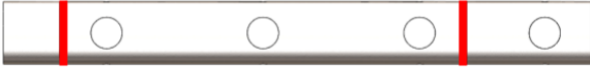
Figure D39: The mounting grooves for the 1/2" retaining rings on the release master, marked in red.
