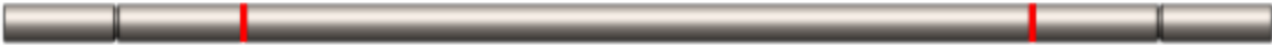
Figure D35: The mounting grooves for the 1/4" retaining rings on the angle shaft, marked in red.
