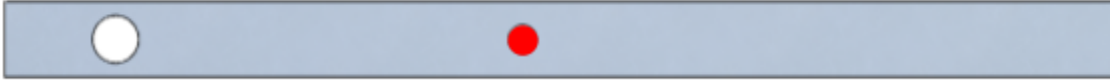
Figure D27: The mounting hole for the 1/4" bushing on stiffener B, marked in red.
