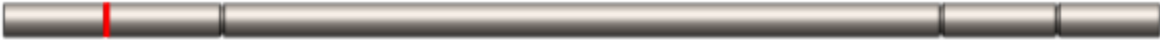
Figure D67: The mounting groove for the 1/4" retaining ring on the angle shaft, marked in red.
