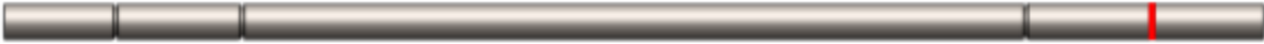
Figure D61: The mounting groove for the 1/4" retaining ring on the angle shaft, marked in red.
