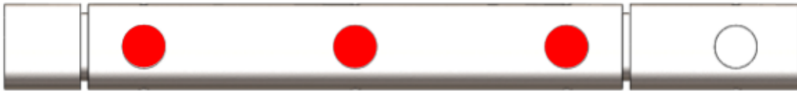
Figure D37: The mounting holes for the release instances on the release master, marked in red.
