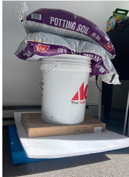
Figure 30: 165 pounds on top of mat, including 80 pounds of soil, 40 pounds in cardboard box of tools, 45 pounds of dumbbells inside bucket for test #2 iteration
