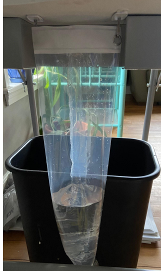
Figure 28: Drape filled with 1000 ml of water attached to the mat with hooks for test #1
