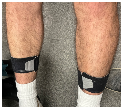
Figure 20b. Movella DOT sensor attached to “patient’s” shins.
