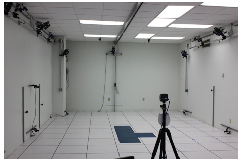
Figure 6: The Vicon infrared marker motion capture system is one of the most popular systems used in laboratory gait analysis ( Mizzou Vicon System , n.d.).
