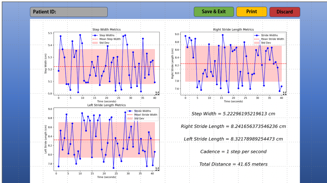
Figure 25e: Representation of the post-trial data screen. This is displayed once the image capturing and post-processing is complete. Physical therapists can print the screen to save data physically, save it & exit from the screen, or discard the trial.
