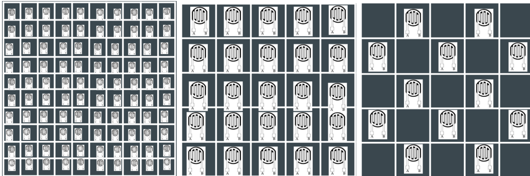
Figure 18: Each visualization represents 5 \times 5 \text{ cm}^2 configuration. On the left is the 4 sensor per \text{cm}^2 configuration which is the gold standard on the market today and the middle configuration is the 1 sensor per \text{cm}^2 configuration that produces not as accurate data but is still suitable for a lot of uses. Finally on the right is the alternating sensor configuration that would cut our costs in half and provide sufficient data to measure step width.
