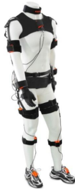
Figure 4: The Xsens MVN is a wearable system containing 17 IMUs placed along the body to track six degrees of freedom ((Muro-de-la-Herran et al., 2014)).
