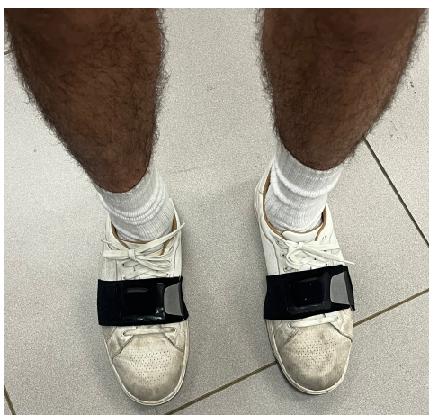
Figure 20a. Movella DOT sensors attached to “patient’s” shoes.
