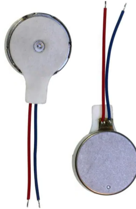
Figure 33. Solarbotics VPM 2 Coin Motor. Achieves 200Hz using 3V power supply. 120mA start, 80mA load current. 32 Ohm Resistance.
