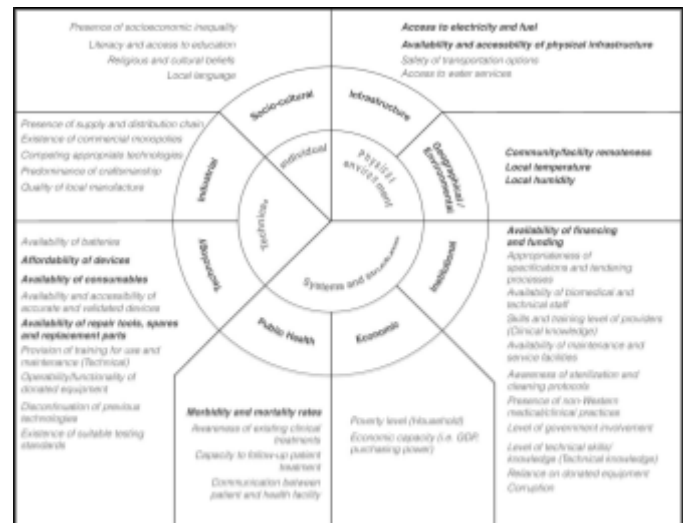
Fig. 4 A visual figure showing 8 different categories of contextual factors applicable for designing for low-resource settings.
