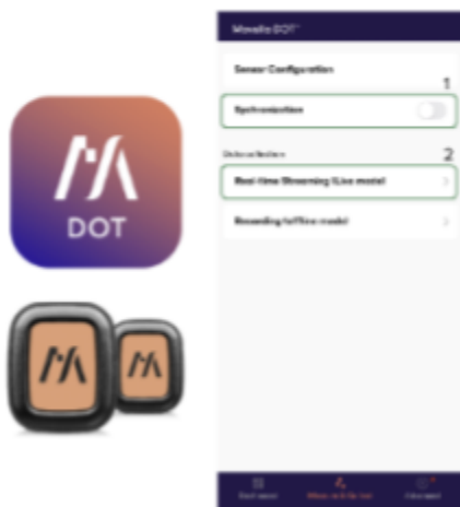
Figure 15. Illustration showing the Movella DOT software and IMUs (left), and the interface of the software which allows synchronization and real time data collection (right)
