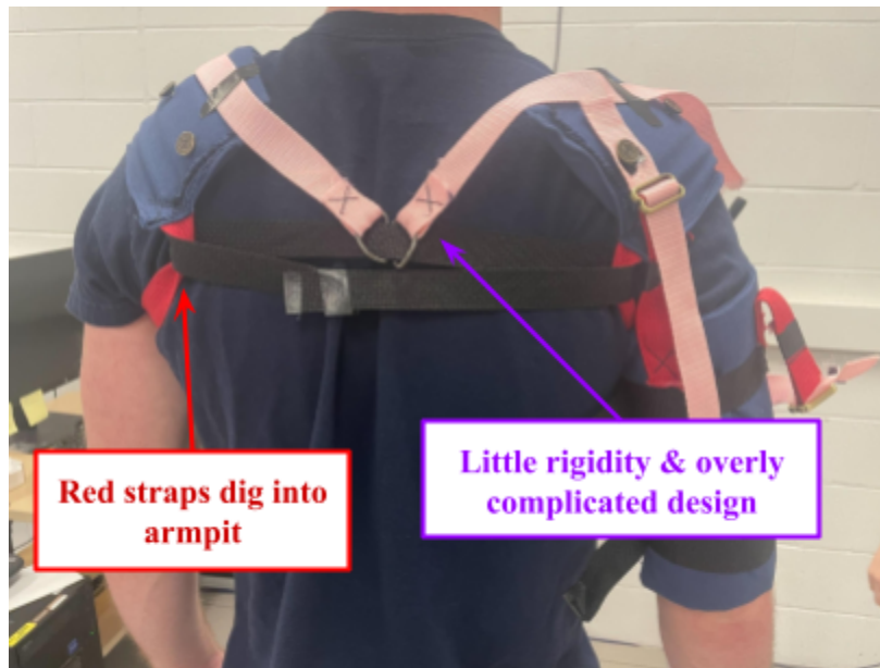
Figure 39: Shows the beta build for the back component with two main issues.
