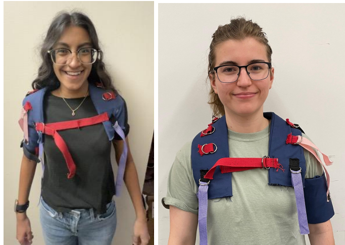
Figure 56: Shows the arm sleeve being worn on both sides of the shoulder pad, meeting the reversible requirements.
