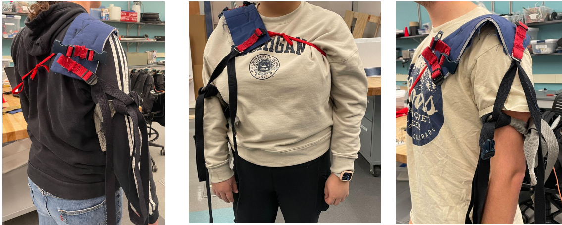
Figure 45: Shows the three participants with the mock shoulder pad with the different types of fasteners. Attached is the black strap that connects to the various attachments and is held together by the wide grey strap that simulates the arm sleeve.
