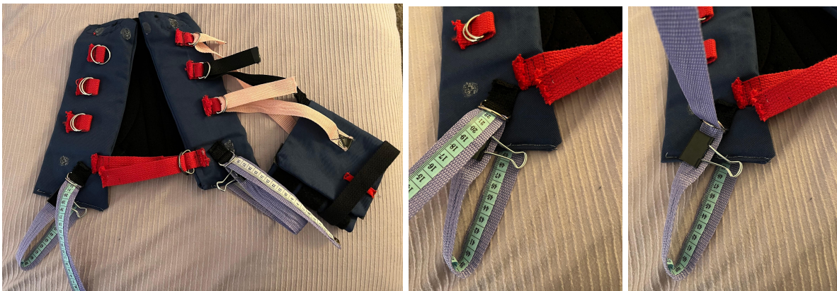
Figure 60: Design with implementation of additional changes. To start, measuring tape was glued onto the inside of the purple straps and binder clips were used to act as hardstops.
