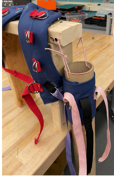
Figure 57: Simulated torso and shoulder joint before test was performed, showing the elastic cord holding up the simulated arm
