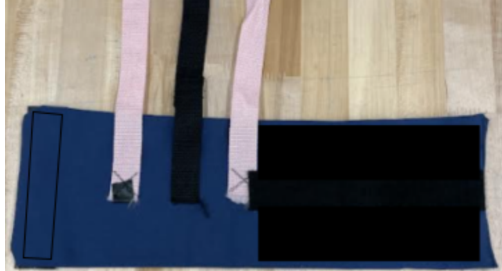
Figure 37: The arm sleeve is 5x15 inches (127x 381 mm). The soft side of the Velcro is applied in a 5x7 inch (127 x 177.8 mm) square with a 2x5 inch (50.8x127mm) of rough Velcro on the opposite side of the sleeve. The three straps are sewn on the sleeve 1 inch (25.4mm) apart.
