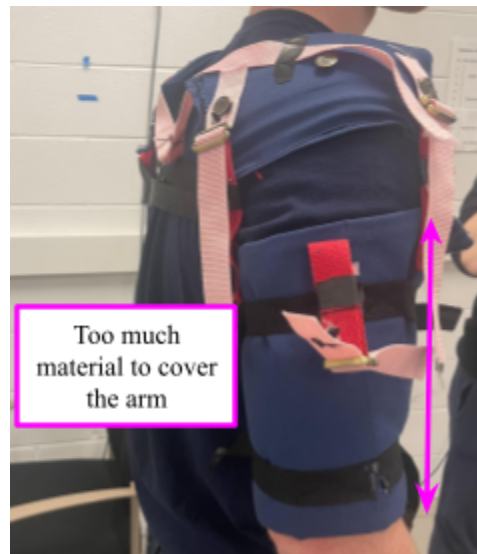
Figure 35: Shows the build beta design for the arm sleeve. The arm sleeve covers too much of the arm, utilizing excessive material.
