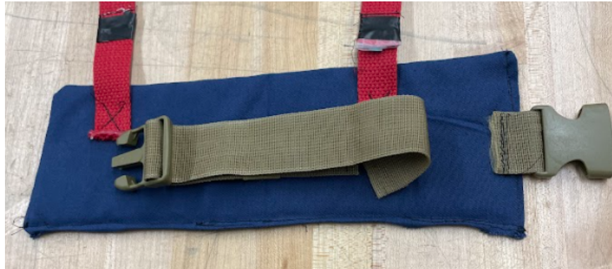
Figure 36: Iteration A.1 of the 101.6 mm arm sleeve with a 38 mm buckle. The present issues are the buckle's fastening difficulty and sliding against the sleeve's fabric.
