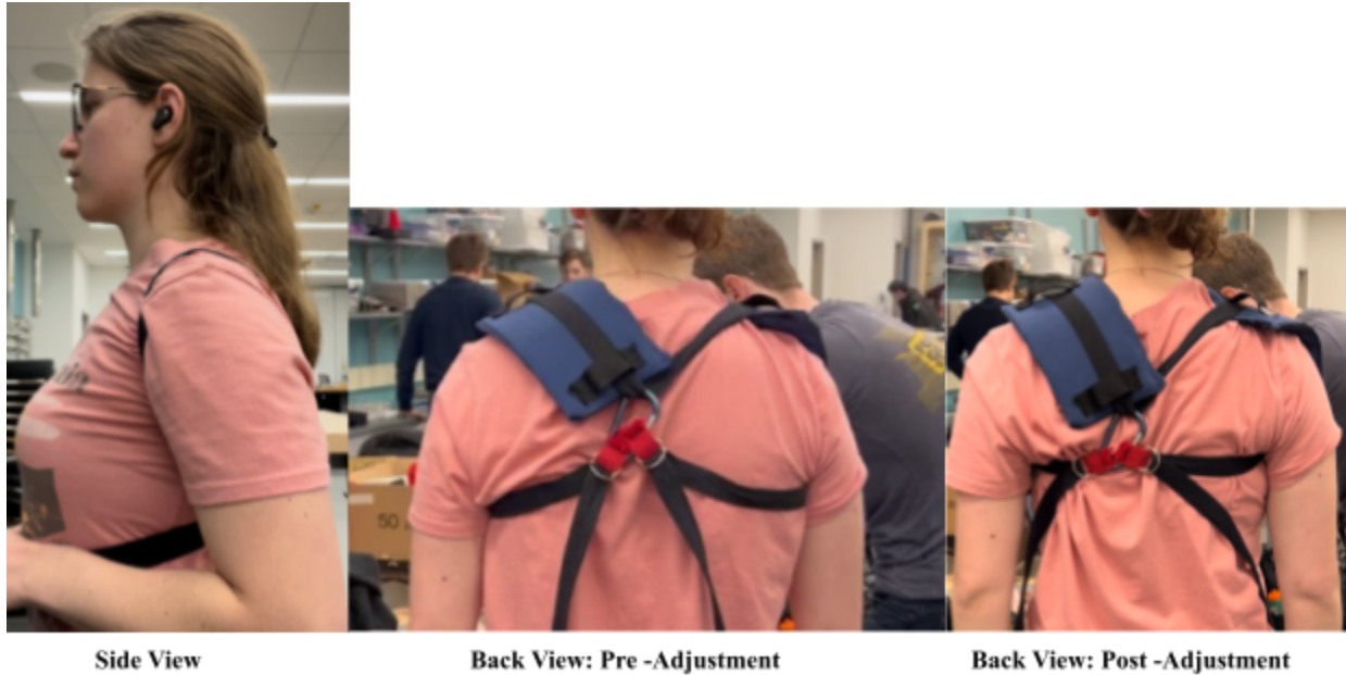
Figure 41: Built prototype of iteration B.1 of the back component pre and post-adjustment where the scapula is pulled back, and the shoulder aligns with the ear.
