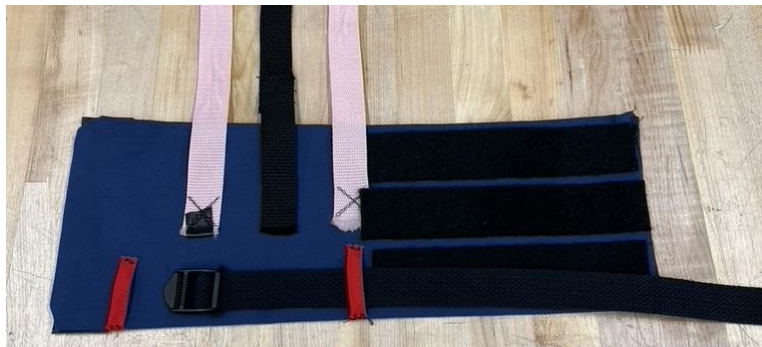
Figure 38: Red belt loops were hand-sewn onto the sleeve to slide the belt and strap adjuster through. The belt is 17 inches (431.8mm) long to accommodate the adjustability specifications and provide enough excess to loop through the adjuster.
