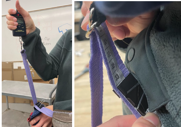
Figure 61: Shoulder pad was secured in a vice, binder clip was secured at a location of 33 cm on the armpit strap, the force gauge attached to the end of the strap. Force was applied to pull and adjust the armpit strap. The maximum force applied was 17.7 \pm 0.8 lbs-f.
