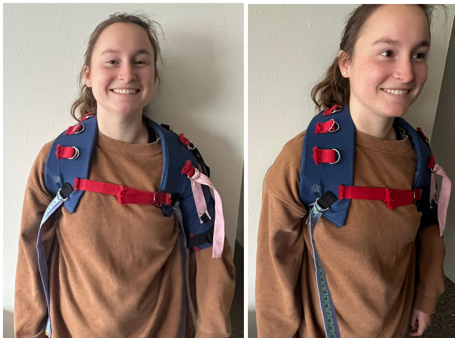
Figure 62: Participants wearing build design with additional changes. Measuring tape is glued onto each strap with a binder clip acting as a hardstop (visible in right picture).
