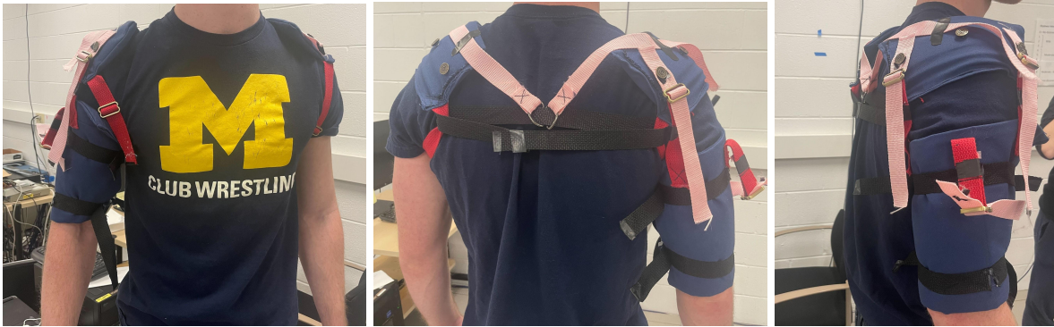
Figure 34: Initial prototype build with multiple issues: the shoulder pads are pulled out of place, bulky/excess material, complicated strap adjustments, and lack of rigidity.
