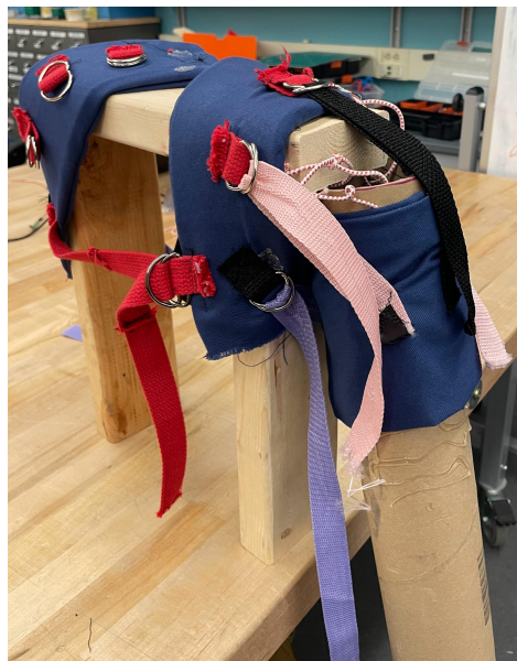
Figure 58: Simulated torso and shoulder joint as test is being performed, showing the simulated arm being pulled up by the device and the elastic cord becoming slack.
