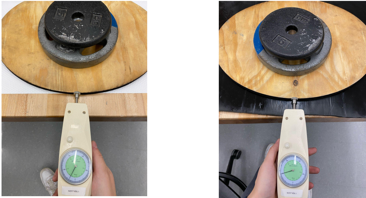
Figure 30. Stability testing setup with thin non-slip kitchen mat (left) and thicker 30-Duro rubber (right)
