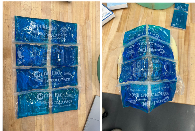
Figure F13. Four gel packs heat sealed vertically (left), gel array over inner components (right)
