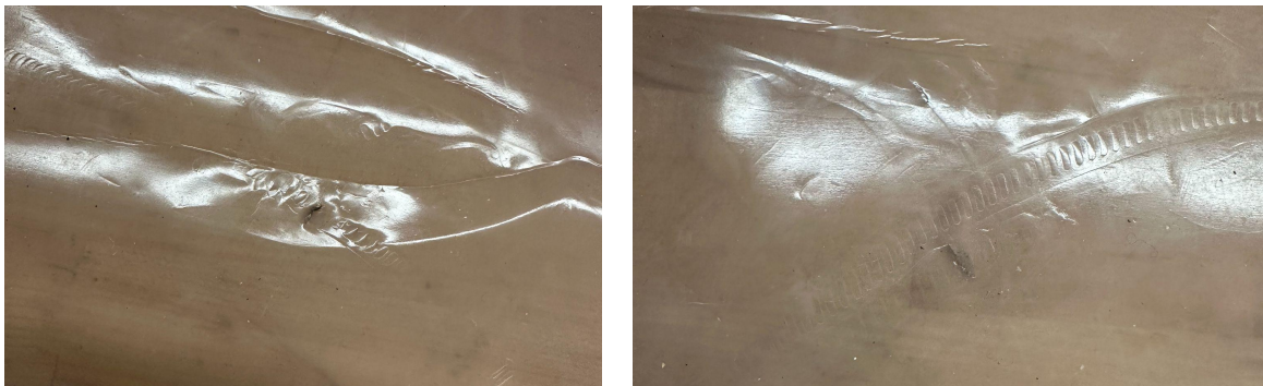
Figure 32. Damage on EcoFlex 00-50 due to hose clamp
