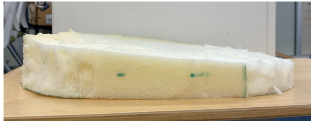
Figure F3. Foam layer side view with 10^\circ angle cut from 3 cm above bottom
