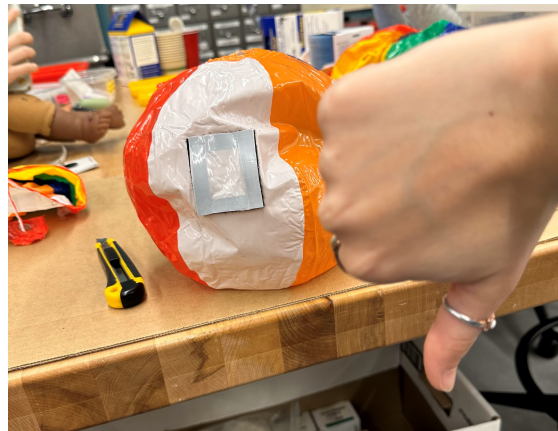
Figure C3. Testing airtightness of velcro flap
