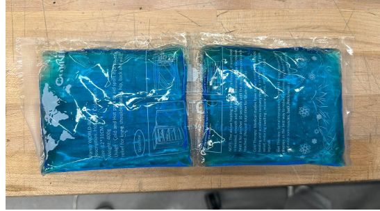
Figure F12. Gel pack, heat sealed down the middle through long edge
