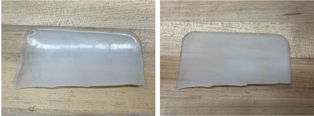
Figure 31. EcoFlex 00-50 sample before testing (left) and after testing (right)
