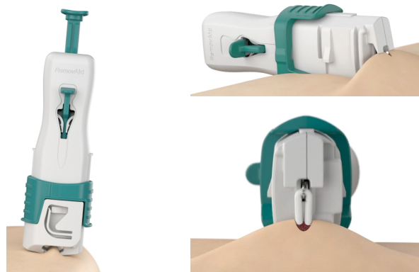
Figure 8. Figure 8a (left) shows the RemovAid making the incision on the arm. The device is then shifted to sit horizontally, where Figure 8c (bottom right) shows the device pulling the implant out by grasping the center of the implant. The location of pulling leads to a higher likelihood of the implant breaking [30].
