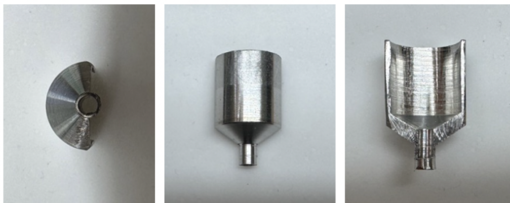
Figure 28. Machined internal device made out of 316 stainless steel.
