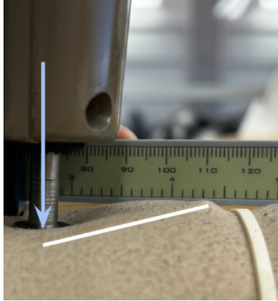
Figure 25. Depth testing test method. The implant was inserted underneath the “skin” and the force gauge pushed down on one end
