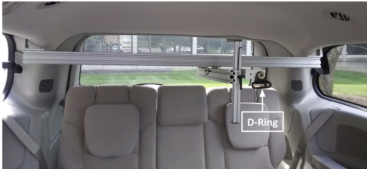
Figure 3: Fixture to allow vertical, lateral, and fore-aft adjustment of D-ring location. Picture taken from original development of the AWTORS [6].
