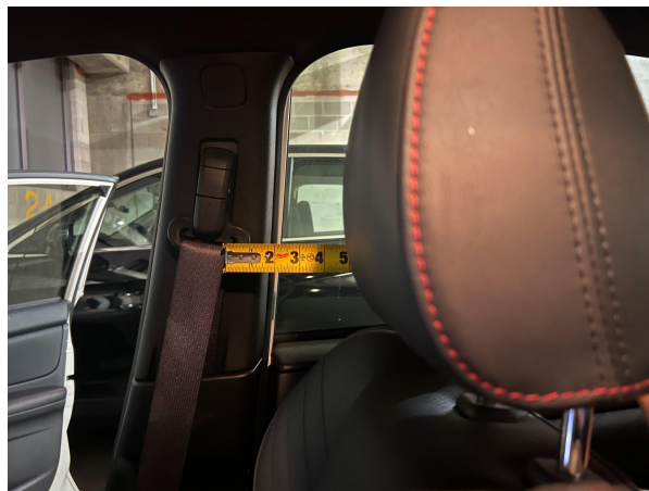
Figure D.3: Aft Distance from D-ring to forward face of seat headrest
