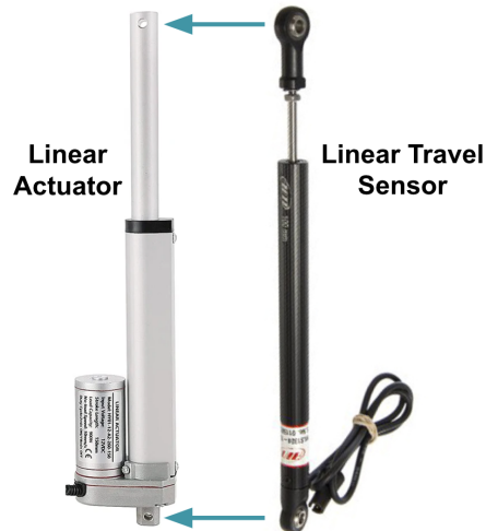
Figure 39: Visualization of how a linear variable displacement transducer could be connected to our linear actuator.
