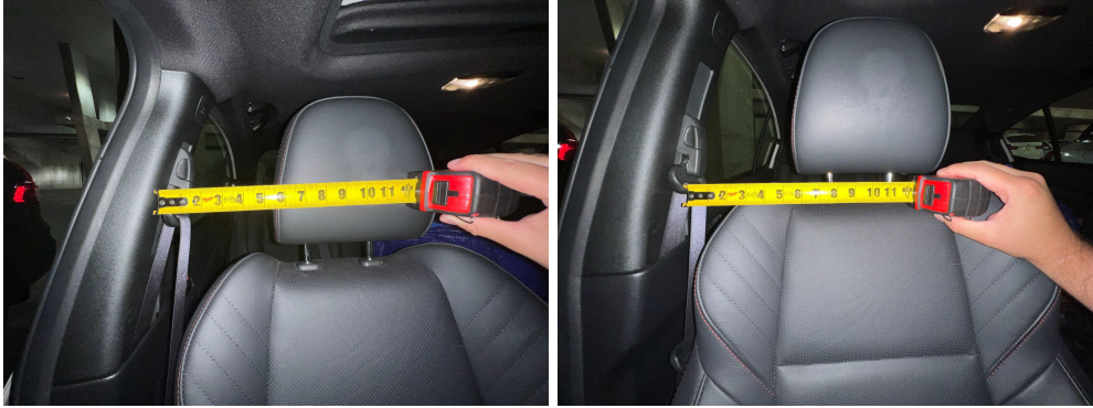
Figure D.2: Inboard Distance from D-ring to centerline of seat headrest with D-ring adjuster in highest setting (Left) and in lowest setting (right)
