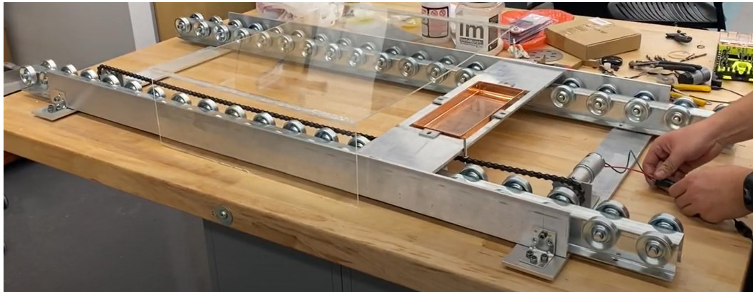
Figure 21: Final build design mechanism, including an acrylic box to model the freeze casting chamber.
