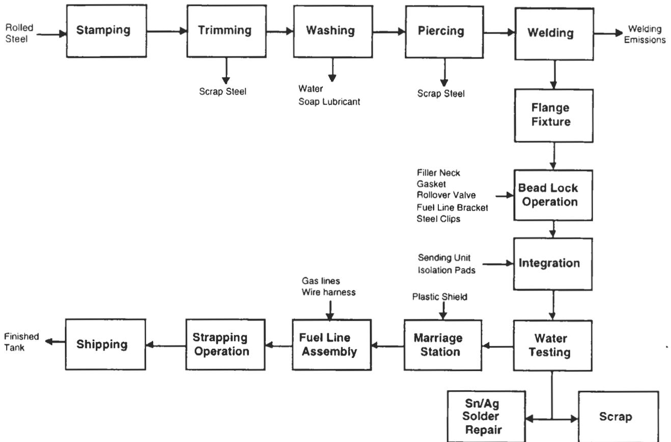
Figure 3-1 Steel Tank Manufacture
