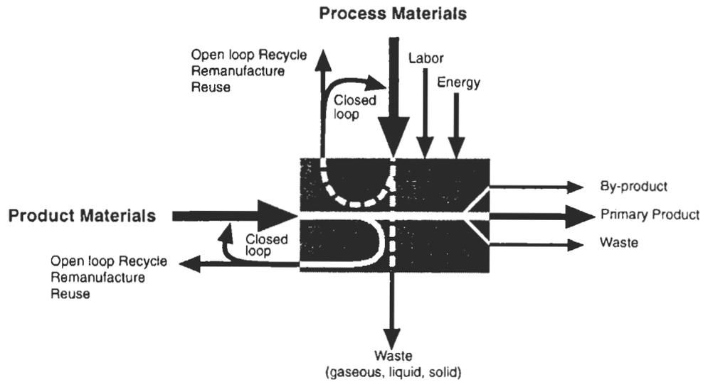
Figure C-2. Flow Diagram Template for Life Cycle Subsystem
