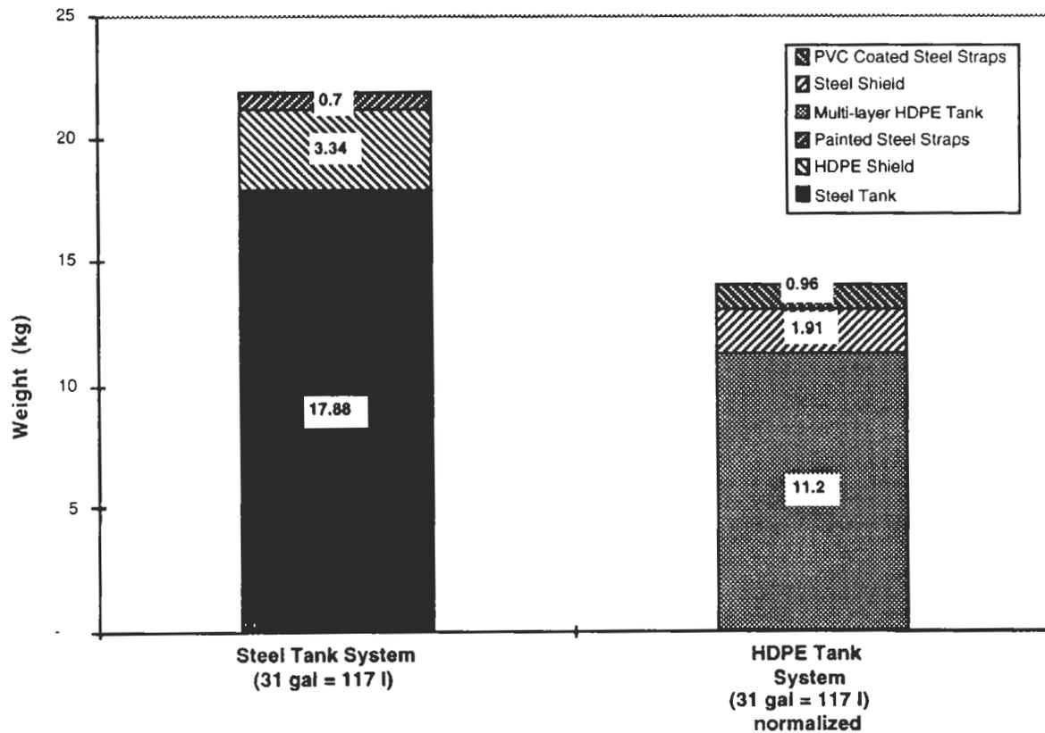
Figure 2-1 Composition of Fuel Tank Systems
